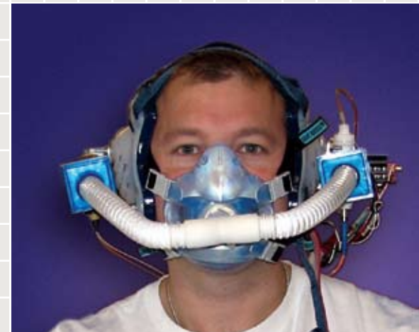
The PUMA (Portable Unit for Metabolic Analysis) is a portable unit that measures crew fitness levels during long-duration spaceflight.
