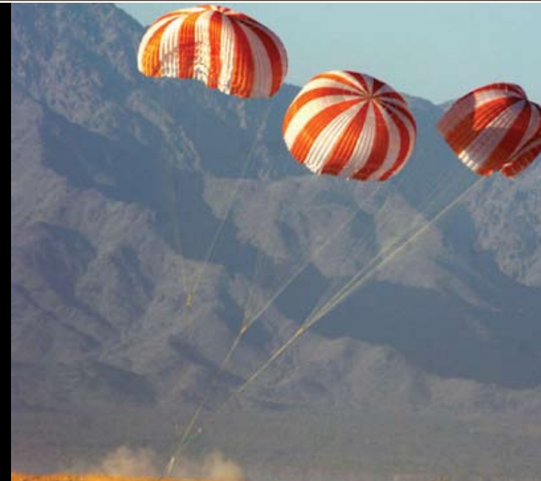
Parachute drop tests are being conducted on the Orion recovery system.
