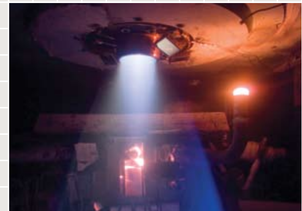
In order to confirm that the heat shield can endure temperatures hot enough to melt metal, testing on the thermal protection system (TPS) occurs inside an apparatus engineers describe as a "room-size blowtorch." In this apparatus, hot hypersonic winds with temperatures that exceed those at the surface of the Sun are created to simulate the heat of reentry.
