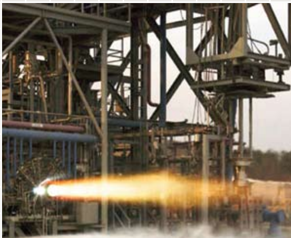
NASA engineers have successfully completed testing of subscale main injector hardware, an early step in development of the RS-68 engine that will power the core stage of Ares V.
