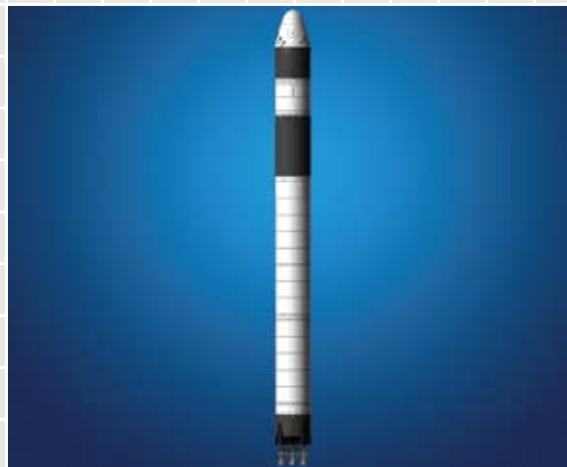
Capable of lifting over 61,000 pounds to low-Earth orbit and over 26,000 pounds to geostationary transfer orbit, the Falcon 9 Heavy from SpaceX will compete with the largest commercial launchers now available.
