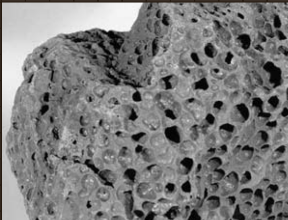
The vesicular nature of this lunar basaltic sample that was retrieved during the Apollo-15 mission leads scientists to infer the presence of gases or water vapor on the Moon. The possible presence of water is one of the factors that will determine the future location of the lunar outpost.
