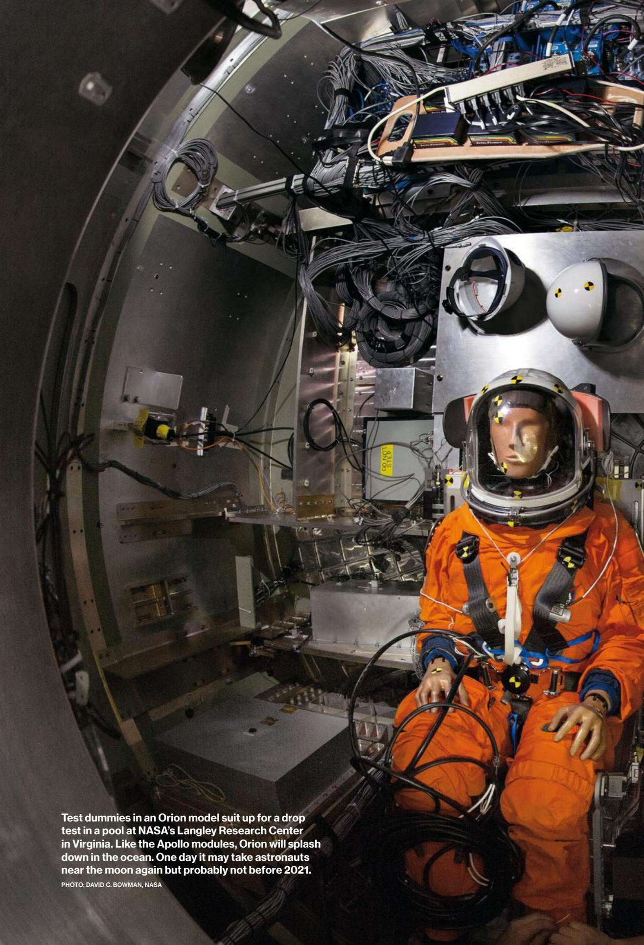
Test dummies in an Orion model suit up for a drop test in a pool at NASA's Langley Research Center in Virginia. Like the Apollo modules, Orion will splash down in the ocean. One day it may take astronauts near the moon again but probably not before 2021.
