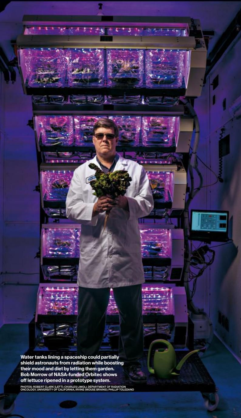
Water tanks lining a spaceship could partially shield astronauts from radiation while boosting their mood and diet by letting them garden. Bob Morrow of NASA-funded Orbitec shows off lettuce ripened in a prototype system.
