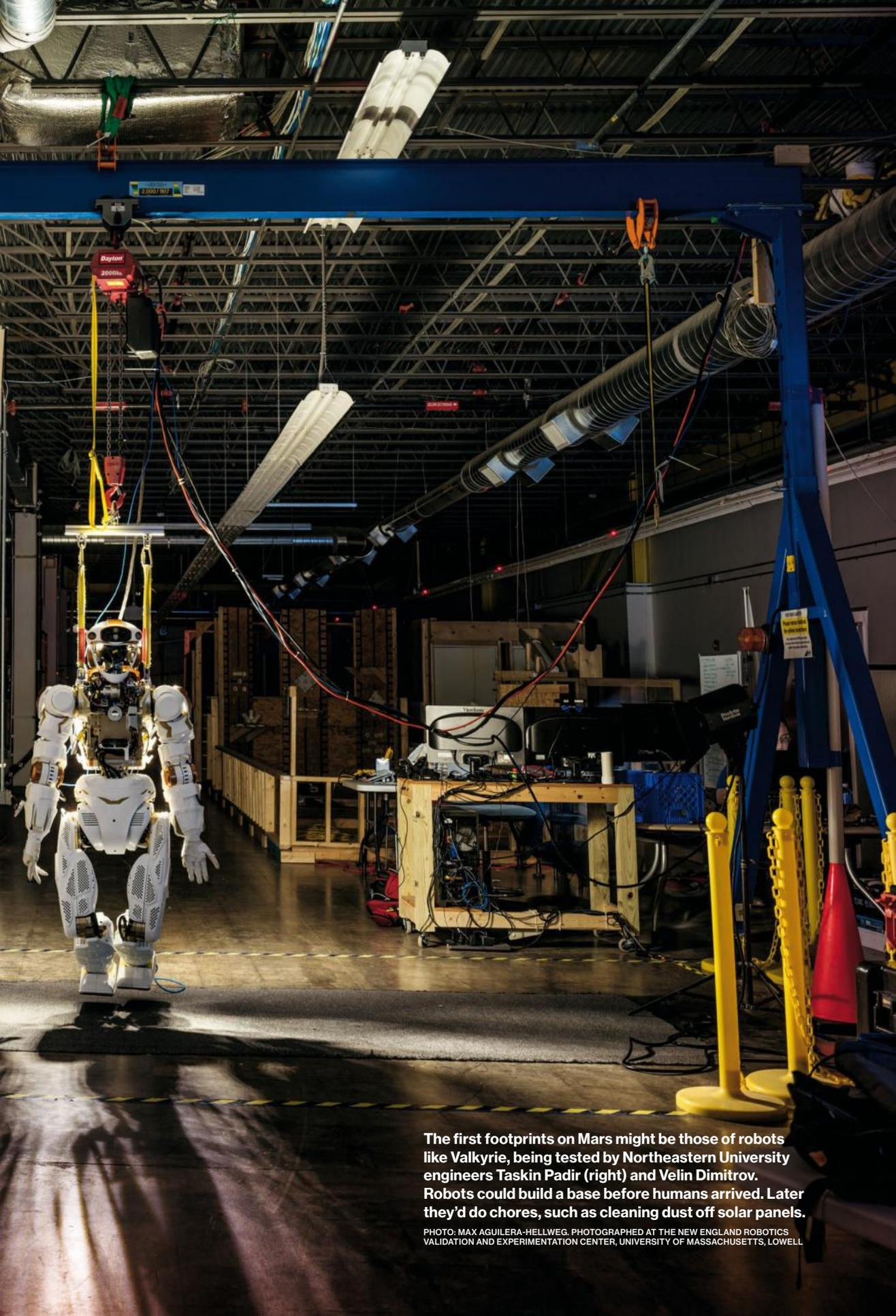
The first footprints on Mars might be those of robots like Valkyrie, being tested by Northeastern University engineers Taskin Padir (right) and Velin Dimitrov. Robots could build a base before humans arrived. Later they'd do chores, such as cleaning dust off solar panels.
