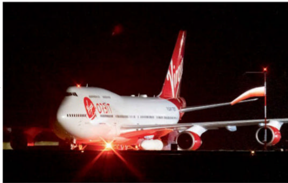
Cosmic Girl (above), a repurposed Boeing 747, carried the LauncherOne rocket (right) tucked under its left wing
