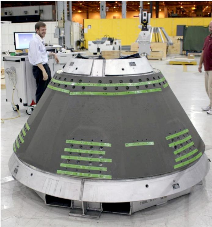
The EFT-1 Launch Abort System Motor Adaptor Truss Assembly (MATA) pathfinder cone is undergoing laser inspections at Michoud Assembly Facility.
