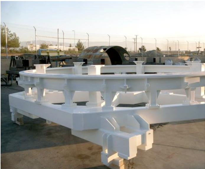
Stringer hole machining on the skin skeleton mate tool structure was completed early along with masking, blasting and painting the tool (photo right). The structure will be transported by Guppy aircraft to Buckley Air Force Base and over to the Denver facility at the end of November.
