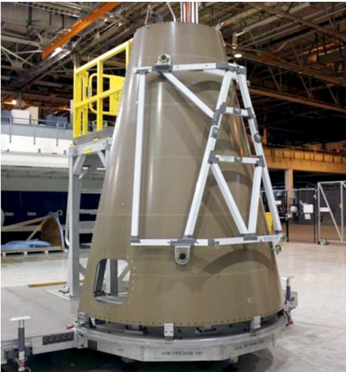
Match drilling and splicing is in process on the two EFT-1 Launch Abort System fillet panels at Michoud Assembly Facility.
