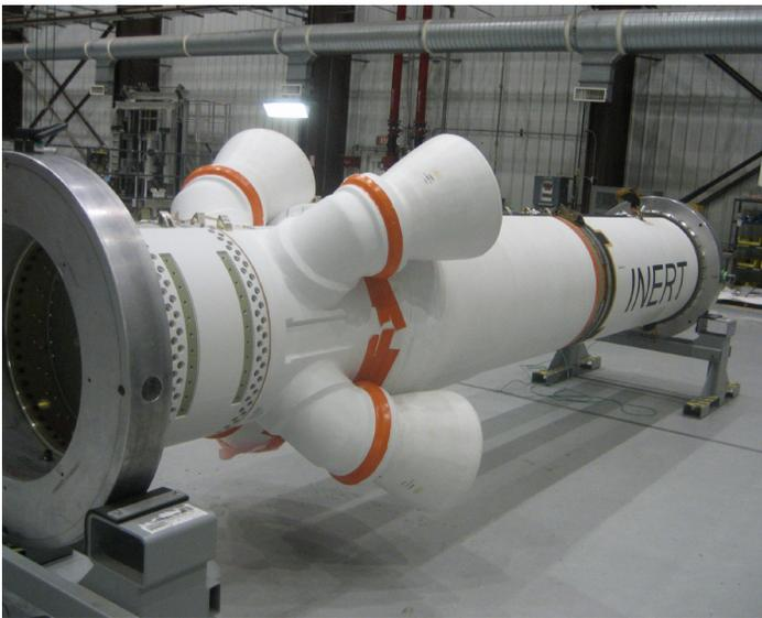
Alliant Techsystems completed development flight instrumentation installation and functional tests for the EFT-1 Launch Abort Motor. Additional EFT-1 operations will continue through February.
