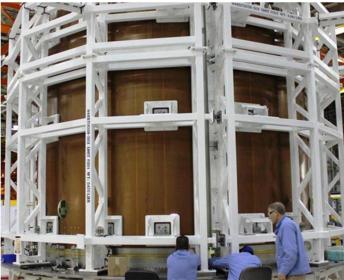
All EFT-1 Service Module spacecraft adaptor jettison fairings have been installed in an assembly tool in preparation for work at the Michoud Assembly Facility.
