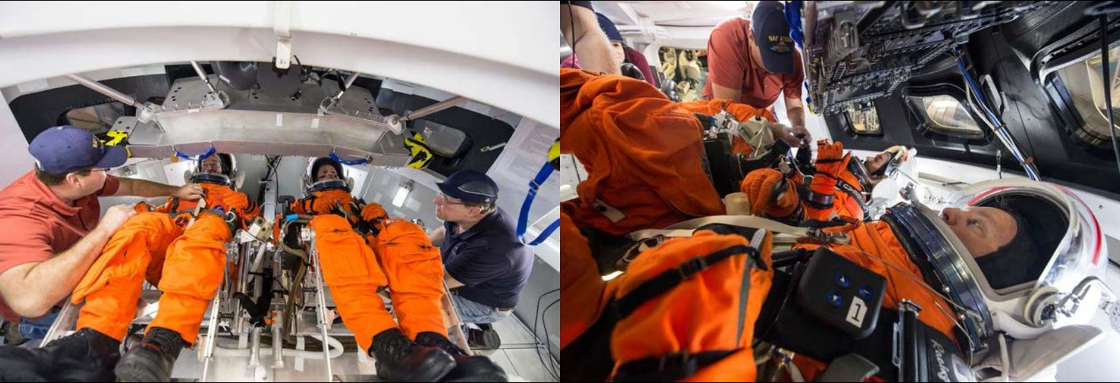
Engineers at NASA's Johnson Space Center in Houston are evaluating how crews inside a mockup of the Orion spacecraft interact with the rotational hand controller and cursor control device while inside their spacesuits. The controllers are used to operate Orion's displays and control system, which the crew will use to maneuver the spacecraft.
