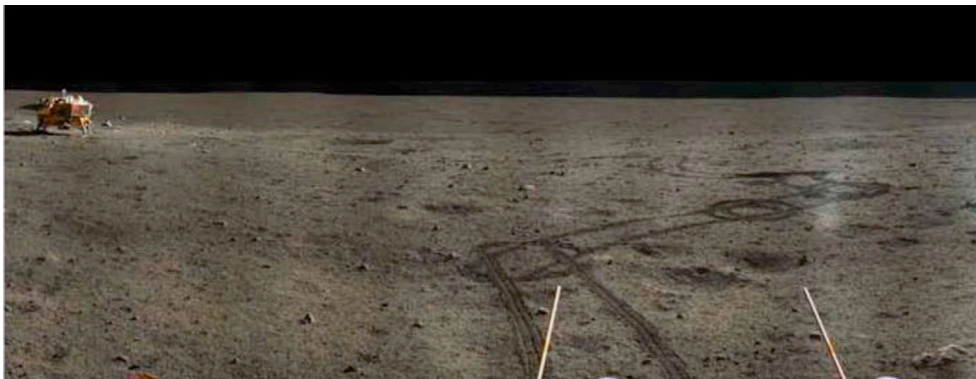
Fig. 1. Lunar surface color panorama obtained by PCAM at exploration. In the background is the lander located to the northeast of the rover, with rover tracks between them visible on the ground. In the foreground are the two antennas of LPR.
