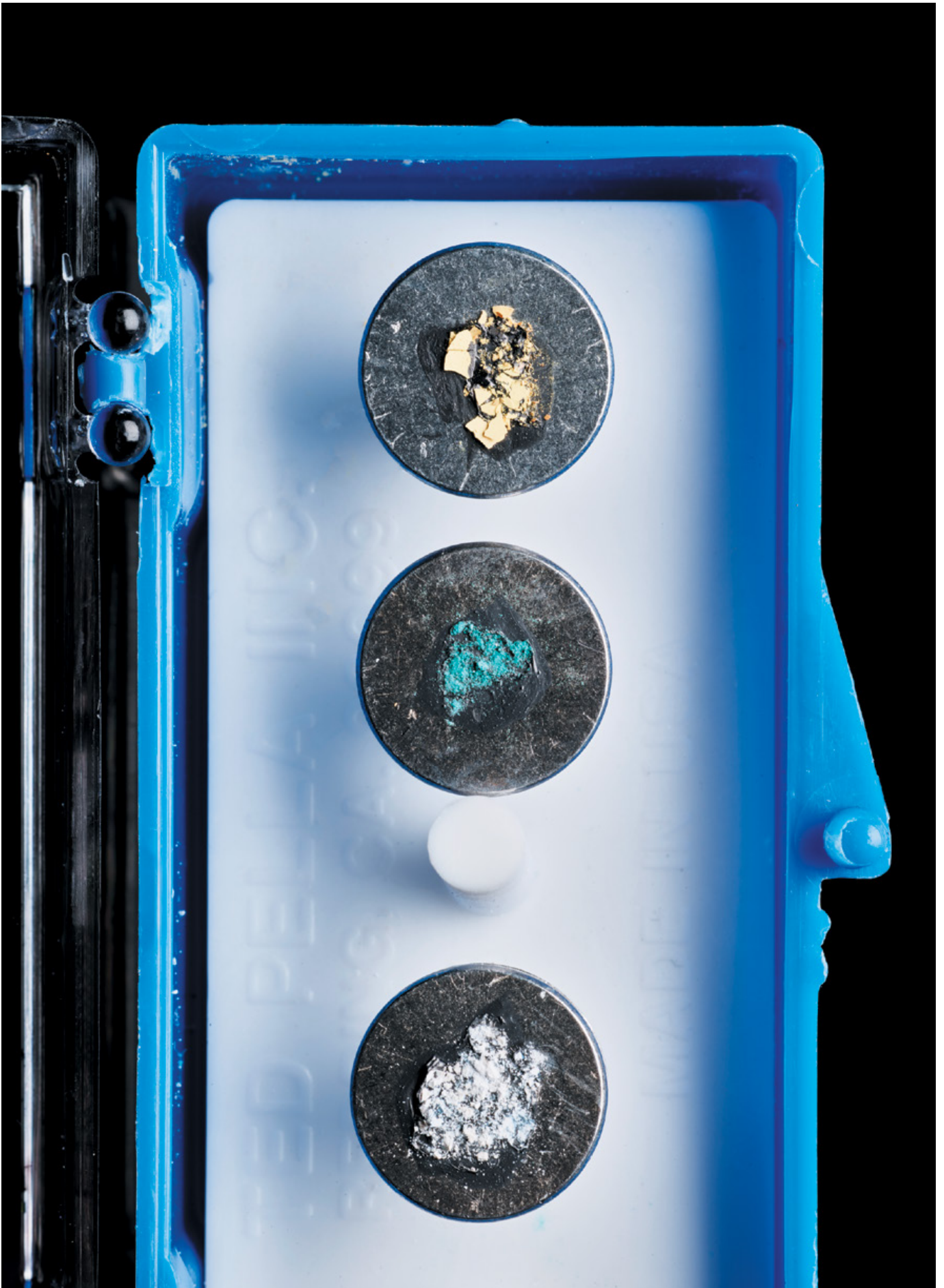
Three samples of metal organic framework crystals are about to undergo scanning electron microscopy. Senesky and her team plan to grow these materials in orbit.
