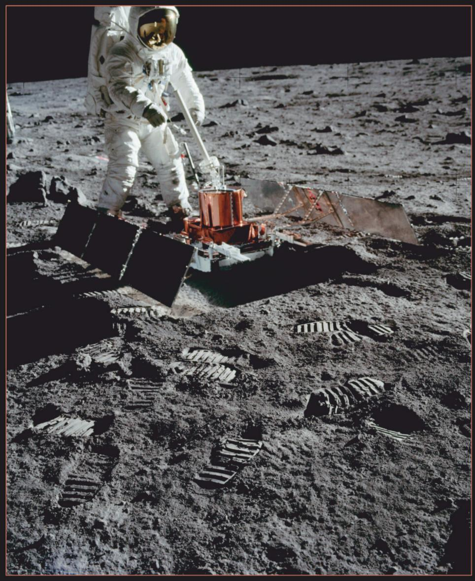
**LUNAR SCIENCE** Apollo 11 astronaut Buzz Aldrin sets up a seismometer on the Moon. The instrument worked for three weeks, detecting moonquakes and gathering information about the Moon's internal structure. Later missions' seismometers transmitted data until 1977.
