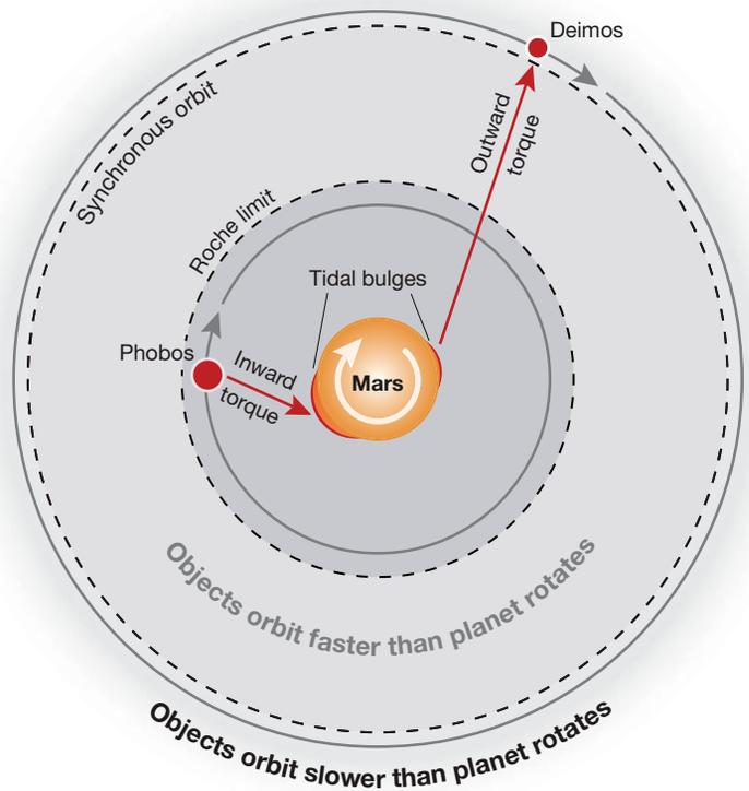
▲ **SATELLITE ORBITS** Deimos orbits just beyond Mars's *synchronous orbit*, the distance at which a satellite's orbital period equals the planet's rotation rate. Inside the synchronous orbit, tides will force massive satellites to spiral in toward Mars; outside it, they'll push the satellite away. Within the Roche limit, Mars's tidal influence will tear the satellite apart.
