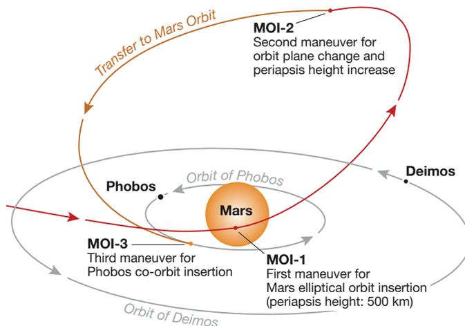
▲ **PLANNED TRAJECTORY** Once Japan's MMX spacecraft enters the Mars system, it will execute a series of maneuvers to insert itself into a *quasistationary orbit* (QSO) around Phobos. A QSO is similar to a geostationary orbit, except that, instead of hovering over the same patch of surface, the satellite moves in a figure eight.
