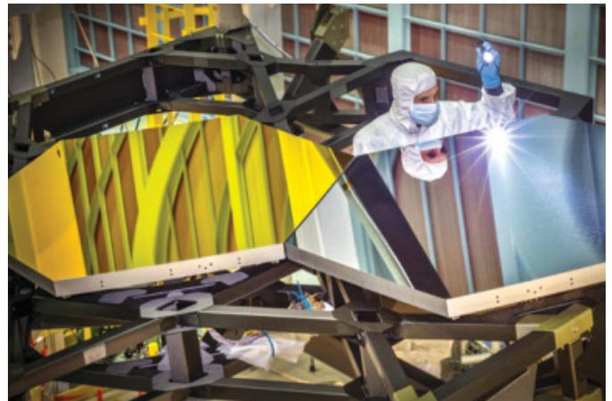
▲ **GO FOR GOLD** An optical engineer examines two test mirror segments, one coated in gold. The frame is a composite material designed to handle Webb's space environment.
