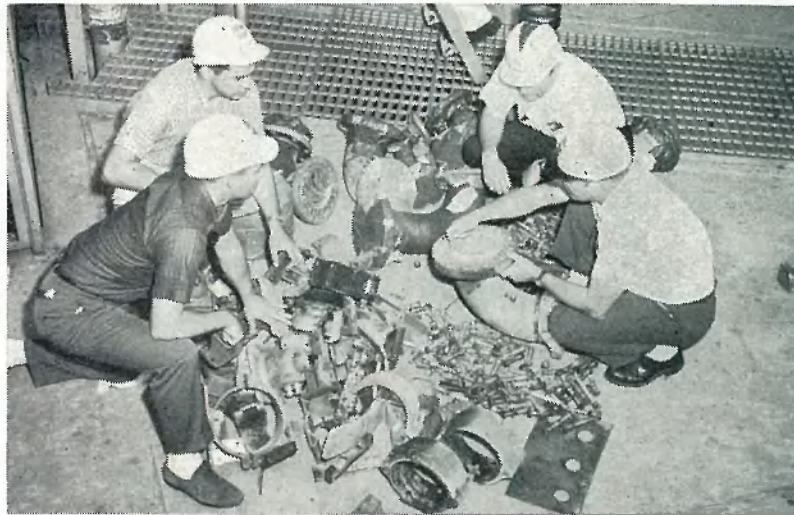
A FEW OF THE several thousand parts that had to be quickly replaced following the recent launch of SA-4 are examined by Complex 34 engineers and mechanics.
