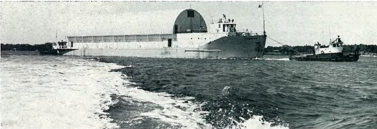
BEING PULLED AND PUSHED simultaneously by tugs, the Saturn barge Promise progresses slowly toward its Cape berth. The vessel moves at about four to six knots in the Intercoastal Waterway.
