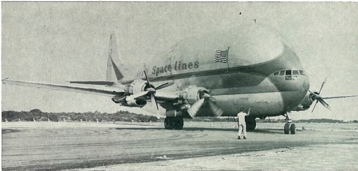
LOOKING LIKE ANYTHING BUT an aircraft, this Aero-Spacelines ex-stratocruiser taxis at Canaveral's skid strip after delivering a dummy S-IV stage from California. The "Pregnant Guppy" can cut delivery time on the S-IV from three weeks to 12 hours.
