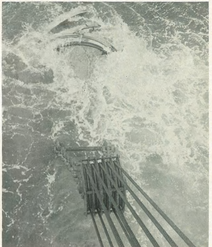
SLASHING THE WATER in a frenzy of motion, the dredge's great cutter head unrelentlessly slices into the river bottom.
