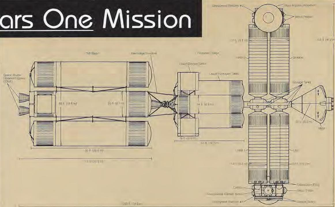
The Mars One Main Ship is a modular structure, consisting mostly of fuel tanks. The crew will ride in the habitability (HAB) modules, each 15.2 meters (50 feet) in length and 4.3 meters (14 feet) in diameter. Tunnels connect the HAB modules with the laboratory and storage modules, and with the Mars Excursion Module (MEM). Drawing: Paul Hudson
