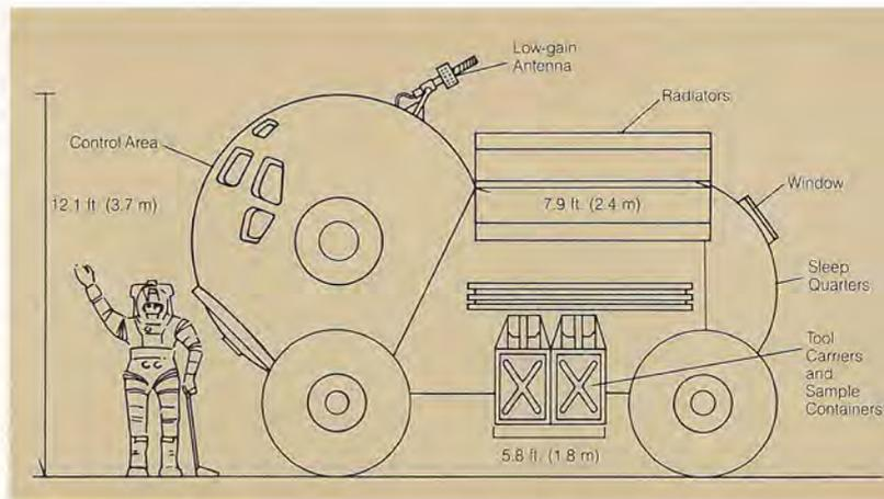
*The Mars Rover is an electric-powered vehicle designed to support a small crew during the long traverse of the martian surface. Like a "recreational vehicle," it provides both transportation and shelter.*
