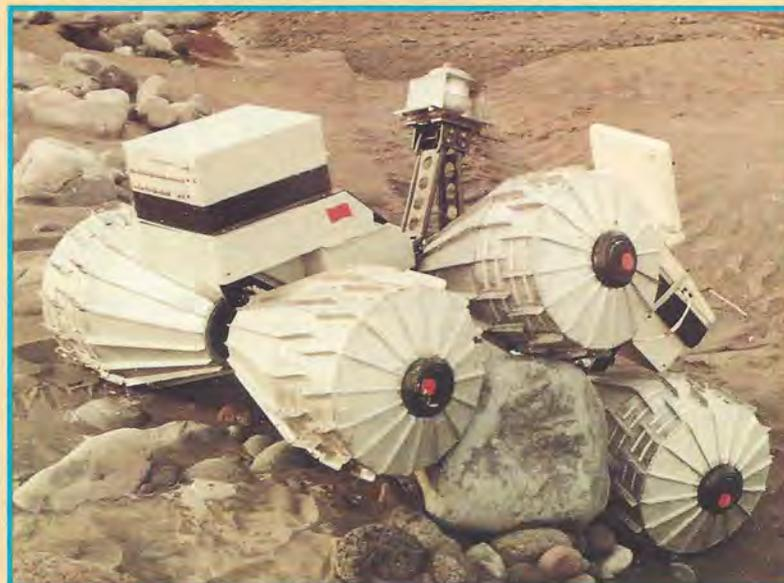
**ABOVE:** The minirover proves that small boulders are no problem as it steps and rolls over this obstacle. This design is a "wheel-walker" and has six conical wheels capable of moving independently in a sort of crawling motion, thus combining elements of both walker and wheeled rover designs.
