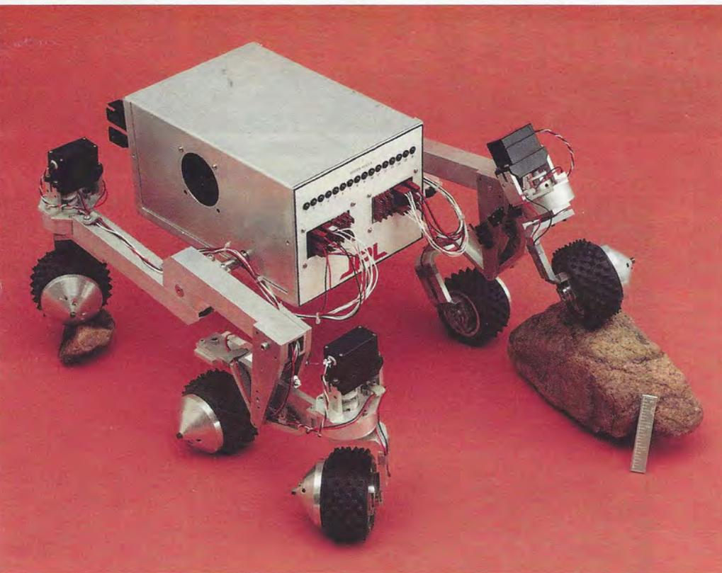
**LEFT:** The prototype Rocker Bogie is able to scale obstacles more than twice a wheel diameter in size (its wheels are five-eighths the size of the Bickler pantograph's). "Rocky" has had a computer brain added and is now being used in field tests as a minirover.
