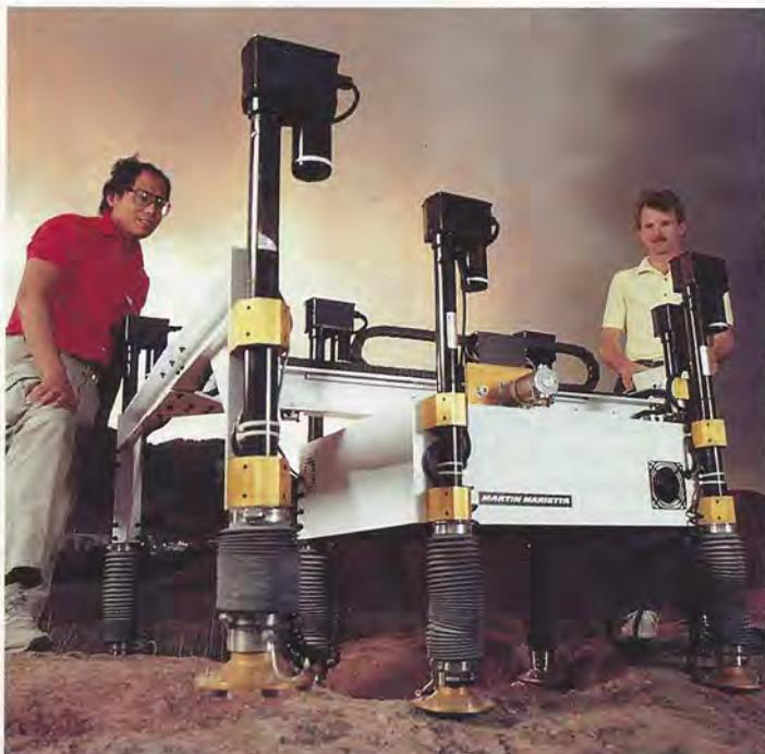
*LEFT: The Martin Marietta Corporation has developed this one-quarter-scale model of the seven-legged "walking beam" to test this rover's ability to climb over obstacles. The model has a four-legged inner platform and a three-legged outer platform. As one platform moves forward, the other remains stationary. Then the moving platform's legs are planted on the ground while the other platform moves forward.*
