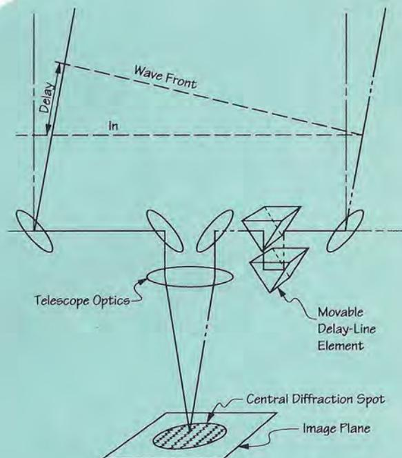
*In a Michelson interferometer, the two beams of light alternately interfere destructively or constructively, giving fringes (bright and dark bands) in the image plane. The path lengths are equalized by delay line optics, giving a very precise measurement of the direction to the source of the waves. Diagram reprinted from TOPS*
