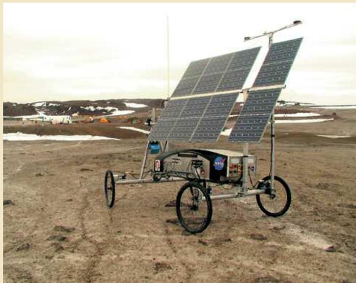
*The "Hyperion" Sun-synchronous robotic rover underwent successful field trials on Devon Island in July 2001, under the leadership of David Wettergreen and Red Whittaker of Carnegie Mellon University's Robotics Institute. Navigating through rock fields and avoiding obstacles autonomously, the rover also managed its power on its own by tracking the never-setting Sun. Hyperion went on circuitous tours several kilometers in diameter and roved 24 hours a day without human intervention.*
