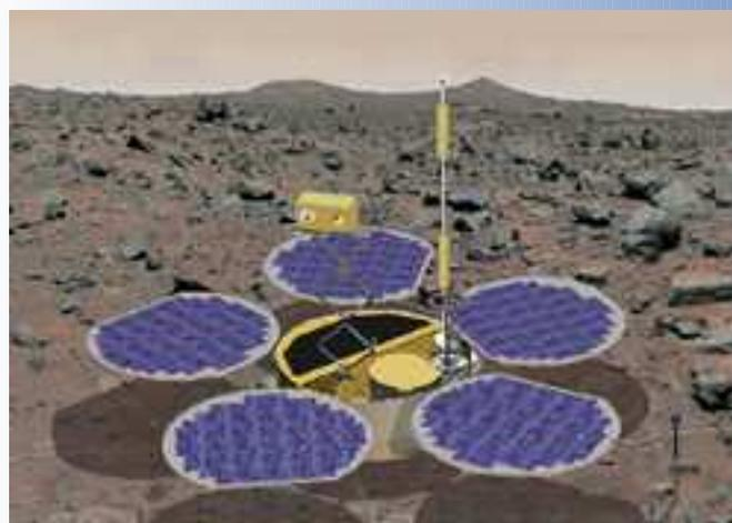
*After touchdown, the PanCam will rise up about 0.5 meter from the main lander deck and, like a little robotic head, will scan the horizon, taking in the sights and sounds of Mars. Illustration: CNES*
