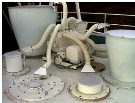
*Various size feeds on top of the GBT's dish receive signals at different wavelengths. The author was relieved to see that each feed had its own snowblower.*
