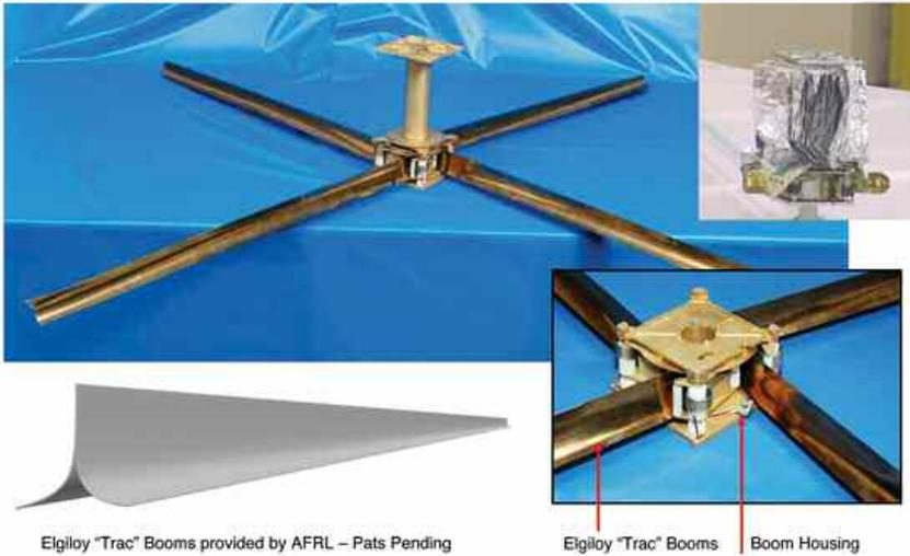
*We've experimented with two designs for the sail's booms and their housing. The first, invented by our team at Stellar Exploration, employed a tape-measure approach to deploy the sails. The second, pictured here, is a Triangular Rollable and Collapsible (TRAC) boom system developed by the Air Force Research Laboratory. Because it is stronger and lighter in weight, we've decided to use this latter version.*
