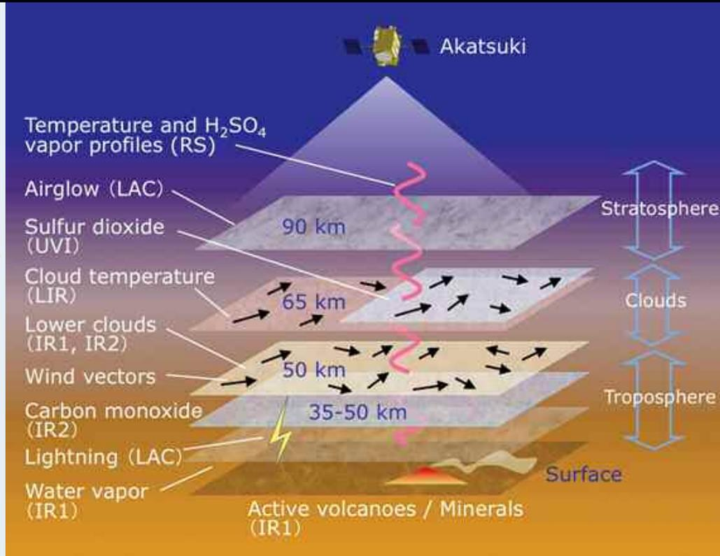
Data from Akatsuki's five cameras—which will include infrared imagery—along with radio occultation measurements will reveal the three-dimensional structure and dynamics of Venus' atmosphere.
