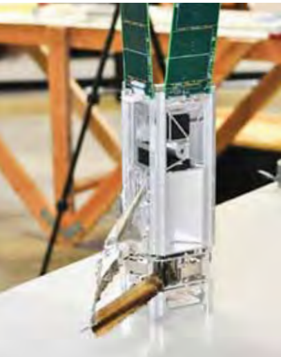
ABOVE LEFT One Mylar sail blade is visible folded into the middle Cubesat unit in the spacecraft's three-unit body. The sail is attached to one of the retractable booms coiled into the bottom unit.
