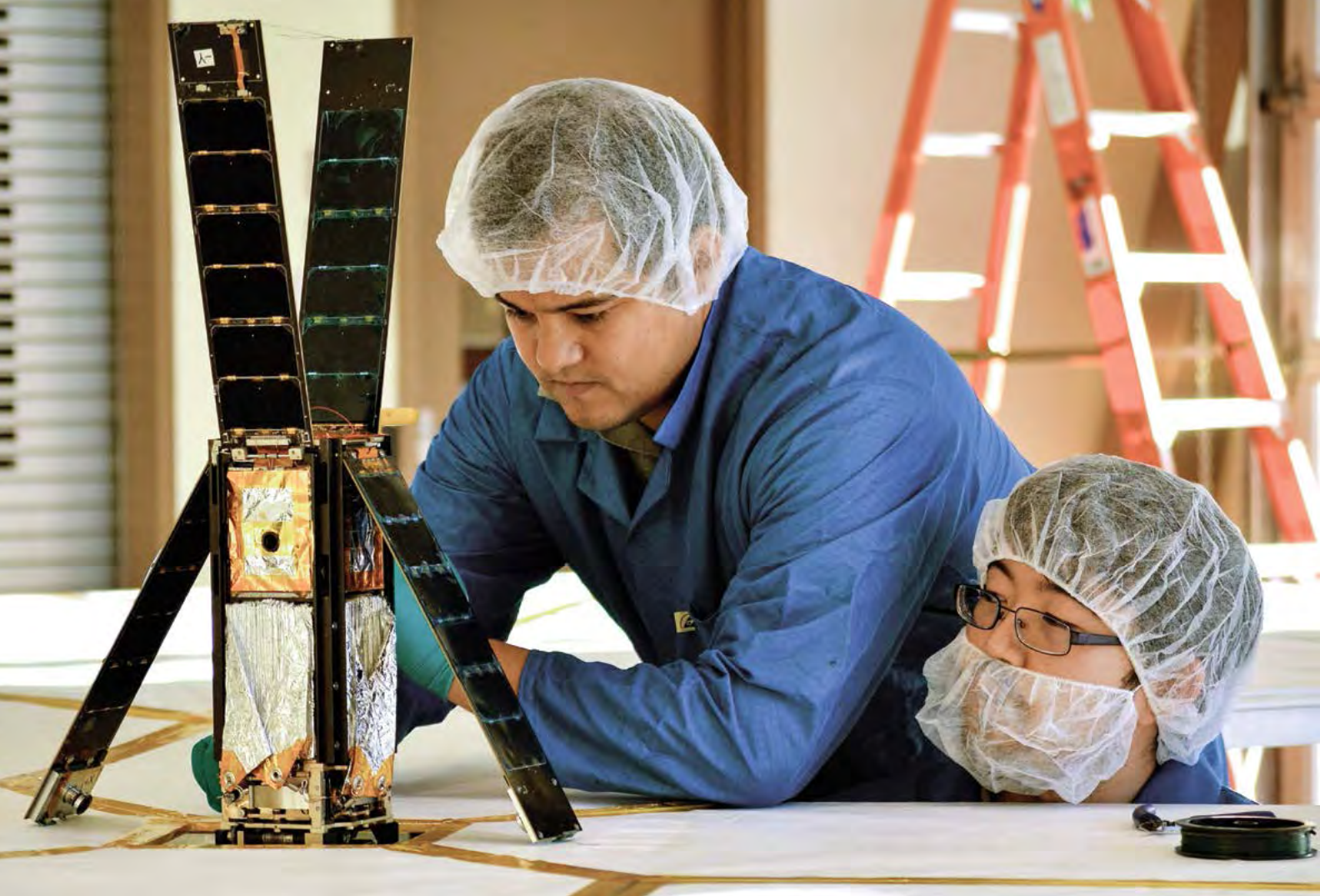
ABOVE At Cal Poly San Luis Obispo, LightSail teammates Alex Diaz and Riki Munakata set up the spacecraft on the deployment table custom-made for LightSail's October 23, 2014 Day-in-the-Life tests.
