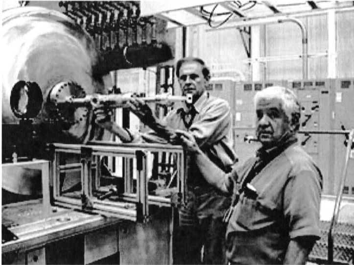
Figure 2-17: Al Reisz (left) and Dr. Jerry Brainerd inspect a small in-space thruster attached to a vacuum chamber. [27]
