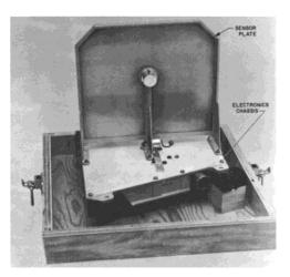
Figure 1–18: Mariner IV cosmic dust detector (picture).
