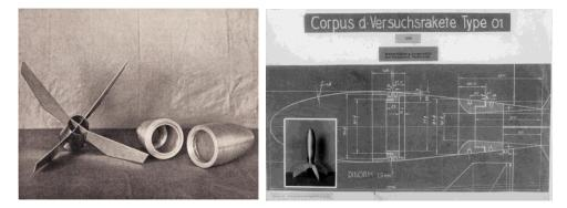
**Figure 1–3 (left)**: Dismantled components of the rocket without propellant. **Figure 1–4 (right)**: Drawing of the body of the experimental rocket type 01.
