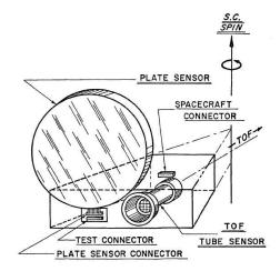
Figure 1–19: Lunar Explorer 35 (IME-E), dust particle experiment (functional sketch).
