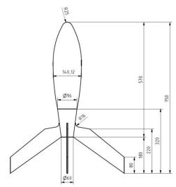
**Figure 1–5**: Reconstruction of Fuchs Experimental Rocket Type 01 by Martin Frauenheim. Drawing by J. Grafe.
