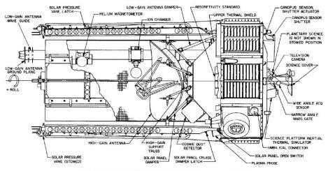
Fig. 2. Spacecraft mechanical configuration: (b) side view, solar panels folded
