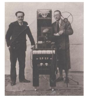
Figure 1–6: Otto Paul Fuchs (right) with the sound recorder Photophon. Austrian patent No. 132981/1932, which was acquired by Klangfilm G.m.b.H. Berlin, a subsidiary of Siemens-Berlin.
