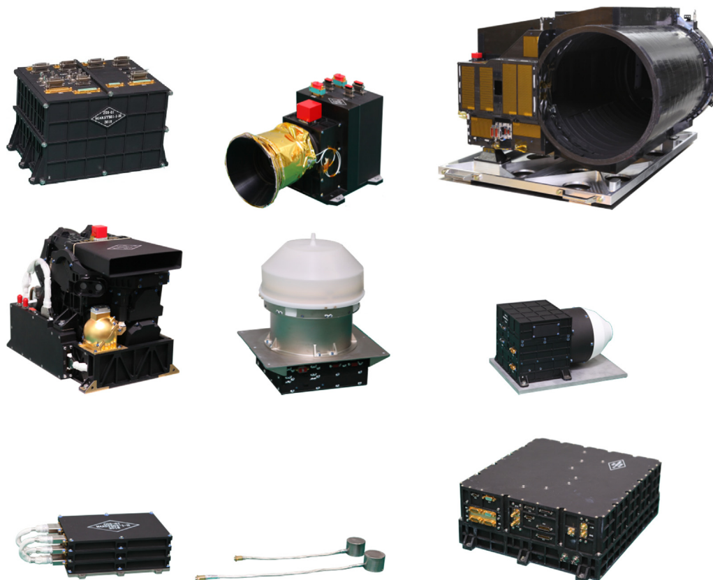
Fig. 5. Pictures of the orbiter scientific payloads (from left to right, first row: payload-controller on the orbiter, Moderate-Resolution Imaging Camera, High-Resolution Imaging Camera; second row: Mars Mineralogical Spectrometer, Mars Ion and Neutral Particle Analyzer, Mars Energetic Particles Analyzer; third row: Electronic equipment and probes of Mars Orbiter Magnetometer, Master processor of Mars Orbiter Scientific Investigation Radar).
