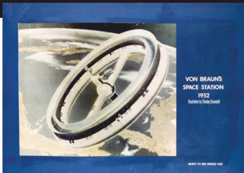
LEFT: In the 1950s, von Braun proposed a ringlike space station, like the one shown in this illustration, that would spin to generate tunable artificial gravity. NASA/MSFC
