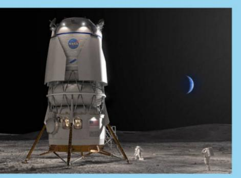
**KITTED OUT.** The 52-foot-high (16 m) Blue Moon will be capable of being loaded with more than 50 tons (45 metric tons) of fuel, and features an upper deck communications array, hydrogen tank, oxygen tank, solar array, docking adaptor, and room for four astronauts. BLUE ORIGIN
