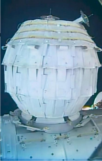
BLOWING UP THE MARKET. Future habitats placed in the shelter of lunar lava tubes could be based on the inflatable BEAM module currently being tested on the International Space Station. NASA
