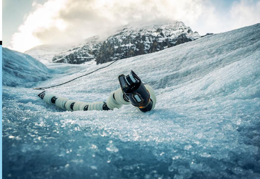
SLITHERING SPEARHEAD. JPL's EELS robot snakes across Athabasca Glacier in Alberta during field testing in September 2023. NASA/JPL-CALTECH
