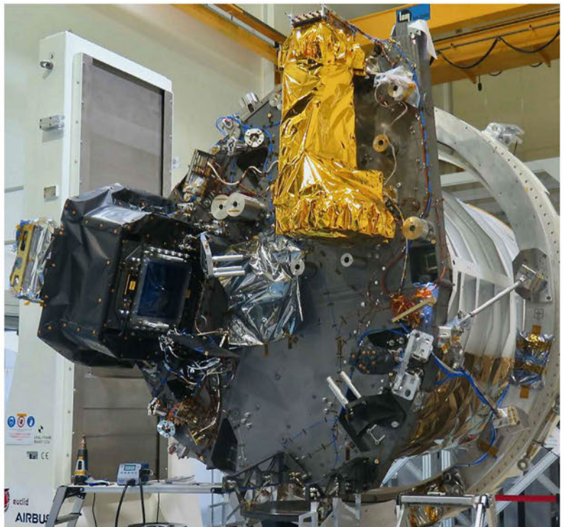
▲ The business end: the visible-wavelength VIS instrument (covered in black insulation) and near-infrared NISP (wrapped in gold insulation)
