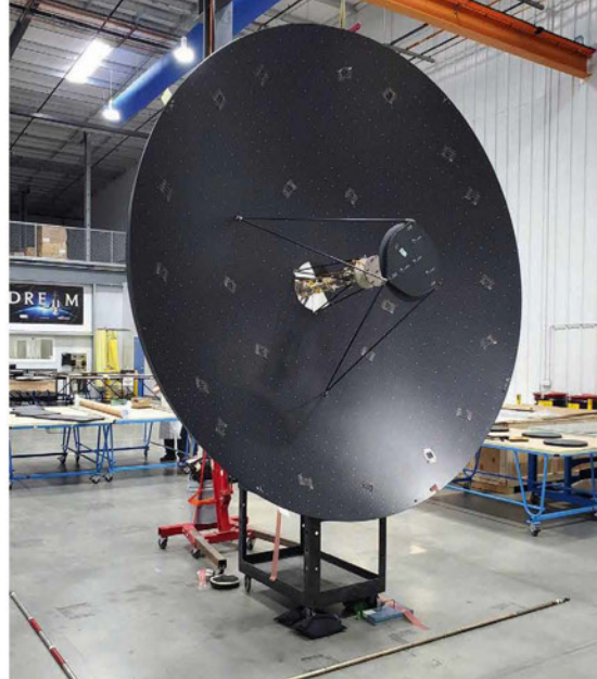
▲ A 3-metre (10ft) high-gain antenna will send data and receive commands from Earth
