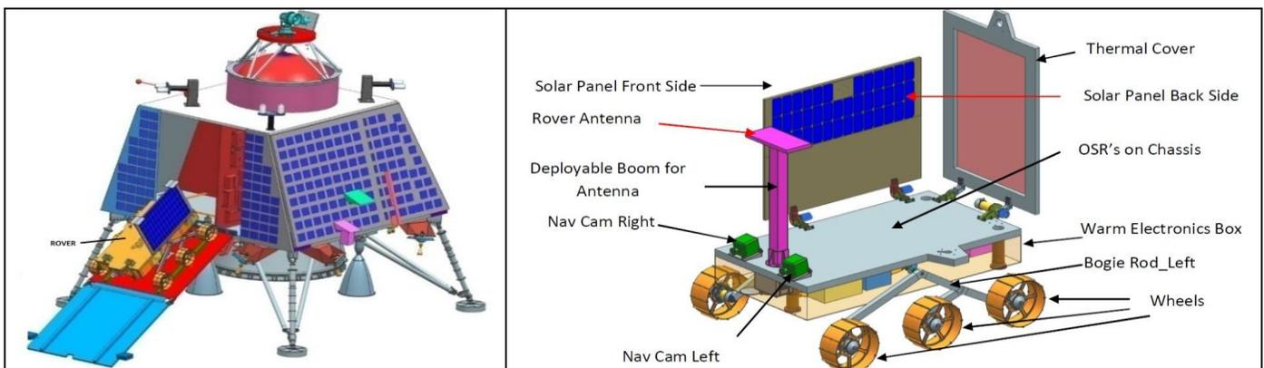
Fig. 2: Schematic of Chandrayaan-2 Lander-Rover Module and Rover in deployed configuration
