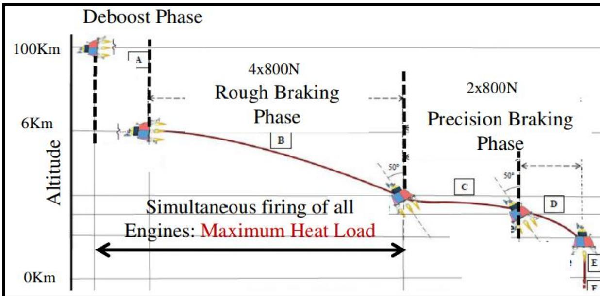
Fig. 4: Chandrayaan-2 Lunar Lander (with Rover) Soft Landing Sequence (Credit: ISRO)
