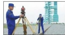
Technicians check a rail used to move rockets on Aug 22, 2020. CAO YAHAO / FOR CHINA DAILY
