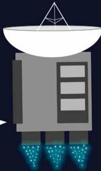
The dream spacecraft would have a nuclear-powered ion engine. Decaying plutonium would provide the power. Ionized xenon gas accelerated through an electric field would provide a weak thrust. The engine could last for years or even decades, allowing for a leisurely but comprehensive tour around an entire planetary system.
