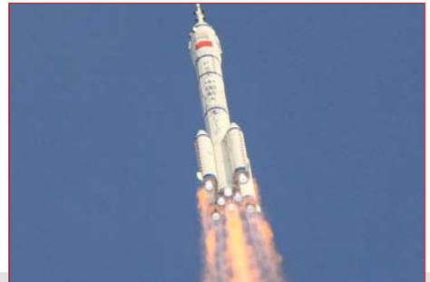
The CZ-2F soared up in the clear sky. Nozzles and flames of the 8 engines are clearly visible in this picture. (credit: Xinhua)
