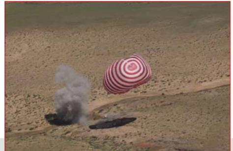
Landing rocket firing and touch-down. Due to strong winds, the capsule did a roll before the parachute was cut. (credit: Xinhua)
