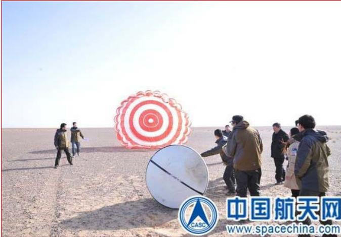
The Chang'e 5-T1 re-entry capsule in an air-drop test. This photo was released in November 2013. (credit: spacechina.com)
