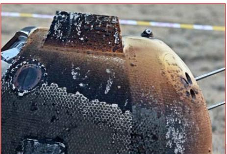
Close-up view of the Xiao Fei capsule. Note stripes in a slightly different colour at the side of the capsule, indicating different ablative materials were used. (credit: Xinhua)
