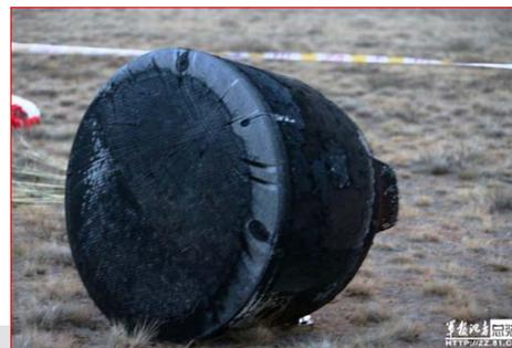
The Chang'e 5-T1 re-entry capsule. This photo shows that its heat shield was scorched much more than its sister Shenzhou. Note that at upper edge of the shield, it was made using a lighter coloured material. (credit: zz.81.cn)
