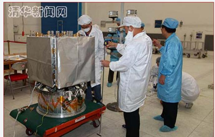
The SCES (Smart Communication Experimental Satellite) in ground testing. (credit: Tsinghua University)
