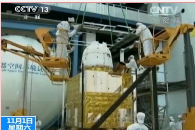
The Chang'e 5-T1 re-entry capsule, integrated with the service module, in final ground testing. (credit: CCTV)
