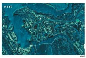
SAR (synthetic-aperture radar) is an active sensing system that illuminates the Earth's surface and measures the reflected signal to generate high-resolution images.
