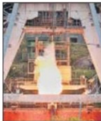
Isro demonstrated successful hot test of the Semi-Cryogenic Engine Power Head Test Article in Tamil Nadu. 1580
