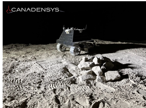
Fig. 1. A prototype of the Canadian lunar rover in a Moon yard at Canadensys.
