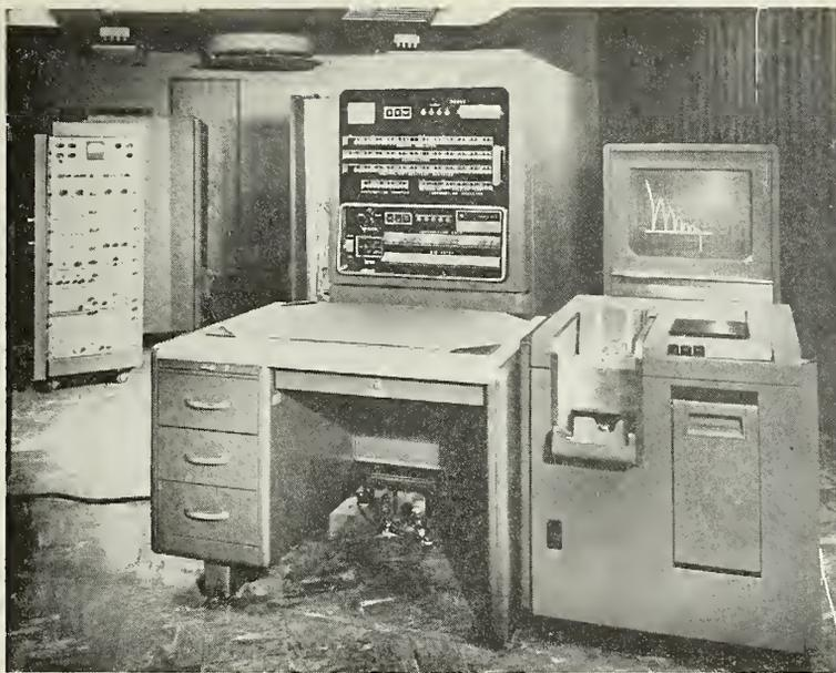
Dr. Paul Herget, Vanguard computation expert, says a cathode ray tube is planned for satellite data display. IBM's 704 Output Recorder was designed for use with a computer. Theoretical path of a bouncing ball is shown.
