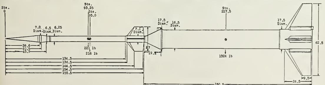
DEACON-NIKE rocket. Accelerometer sphere is located at bulge in *Deacon* immediately aft of nose cone (left).
