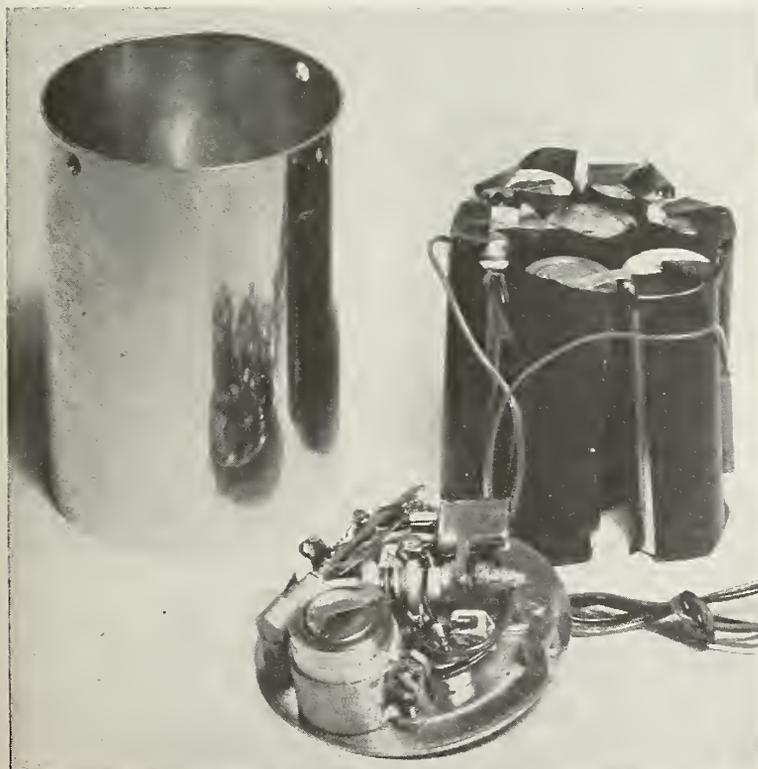
Minitrack transmitter. Circuit assembly in foreground. Batteries at right.
