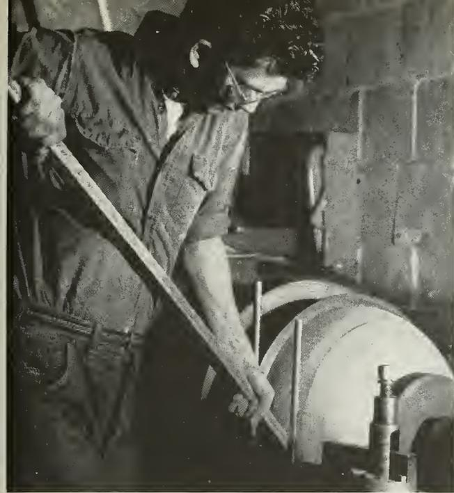
Hours of tedious work go into manufacture of hemispheres which are joined to form 20-inch Vanguard satellite. Sidney H. Braddy, NRL machinist, presses piece of sheet aluminum against large dome revolving in a fast-moving lathe. Metal is gradually worked closer to domed form to produce hemisphere.
