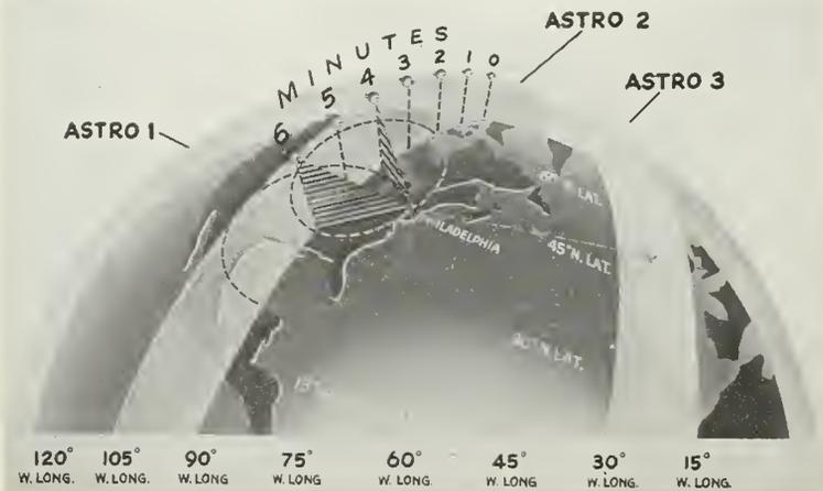
Figure 6—Spherographic technique for positioning a location.
