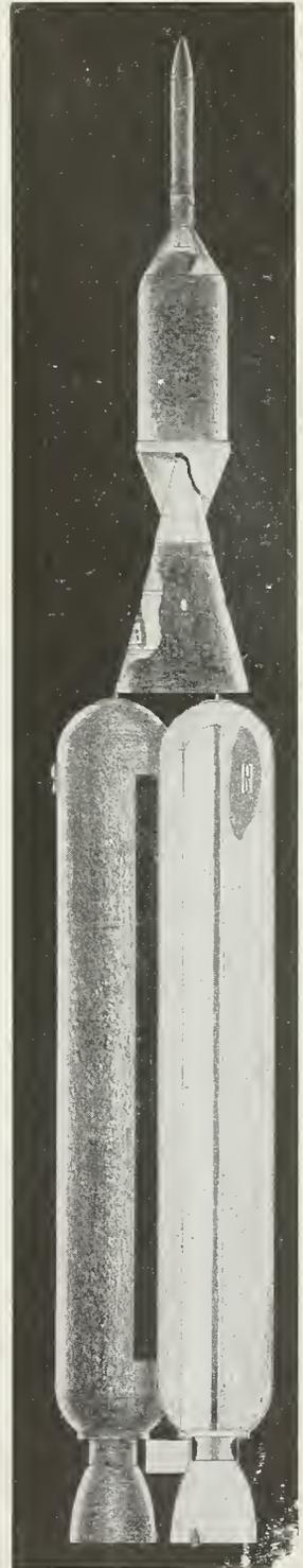
Cross section—vehicle is approximately 35 feet in length. Rockets shown with high drag nose section.
