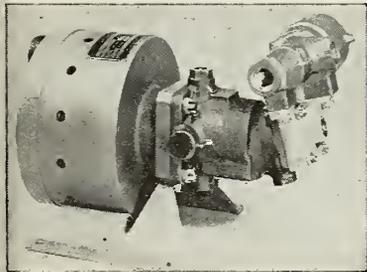
hydraulic motor. Speed control reportedly is within  $\pm$  or  $-2\frac{1}{2}\%$  regardless of load and special adaptations will maintain 400-cycle frequency within  $\pm$  or  $-0.1$  percent.
