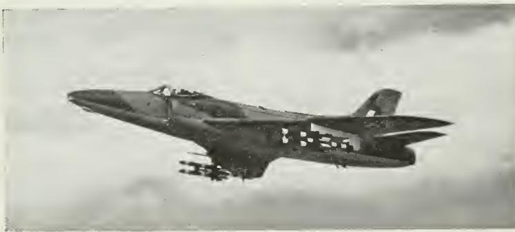
Vickers-Supermarine *Swift* MK7 supersonic fighter, fitted here with two Fairey *Fireflash* air-to-air guided missiles, was unveiled at recent SBAC Farnborough exhibition. It is the second British fighter to mount *Fireflash*, the other being the Hawker *Hunter*.
