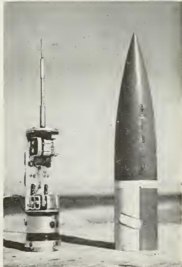
Telemetering unit for Baby rocket.
