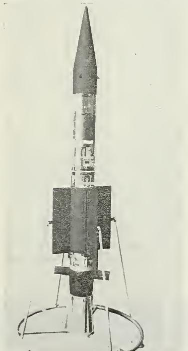
Declassified photo of one of early types of control test vehicle built by Bristol Aircraft Ltd. Maximum velocity exceeds 2,000 ft./sec. Peak acceleration is 35 g's. Triplex tandem boost burning time is two seconds.
