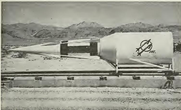
This new rocket sled, built under Army direction by Aircraft Armaments, Inc. reached speed of 1,300 mph during recent tests at Naval Ordnance Test Station, Inyokern, Calif. The 7,000-pound sled, powered by three solid-propellant rockets, reached this velocity in less than 2.5 seconds. This particular test vehicle was designed for the
