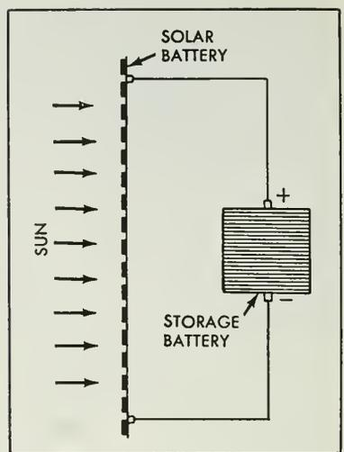
Simple diagram of solar battery principle. This system may be applicable to small, uninstrumented satellites shortly.
