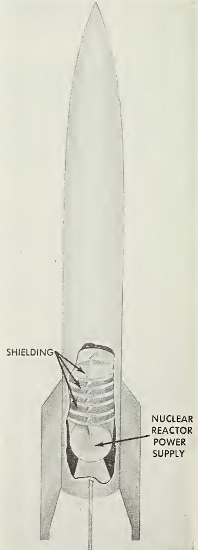
Nuclear reactor power supply sources need only be shielded on the side facing instrumentation or crew compartment.
