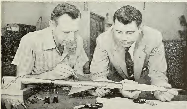
North American engineers ready a model, possibly suggestive of the *NAVAHO*, for wind-tunnel tests. Note the extreme fineness ratio, the delta airfoil on the aft section and the small canard stabilizer close to the nose.
