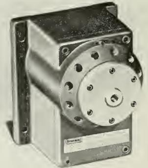
Basic unit consists of a stator having 12 input ports and a rotor that connects any one of these to an output port. A unidirectional high-torque motor rotates the rotor to a desired position and built in provisions are available for indication of position either visually or digitally for operation of recording devices.
