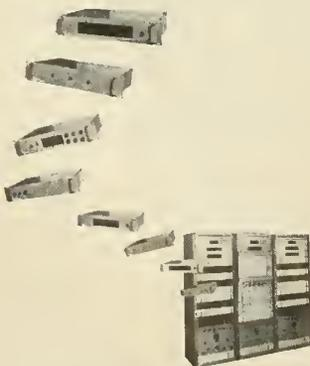
Now from five basic E-I modules, almost any combination of instruments can be assembled for precision, digital measurement of DC, AC-DC, Ohms and AC-DC Ratios. The basic E-I modules never become obsolete. As needs change, simply regroup or add new modules. This new modular concept provides maximum versatility and enables equipment to be kept current at minimum cost and engineering.
