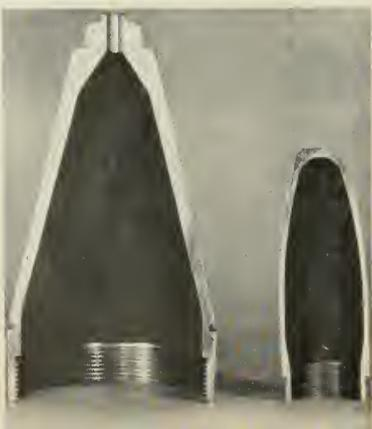
and extrude items with varying wall thicknesses is attracting increased attention from rocket and missile designers. Its cold forming operations extend into the 4130 and 4140 alloy steels as well as in mild steels, aluminum, copper and brass.
