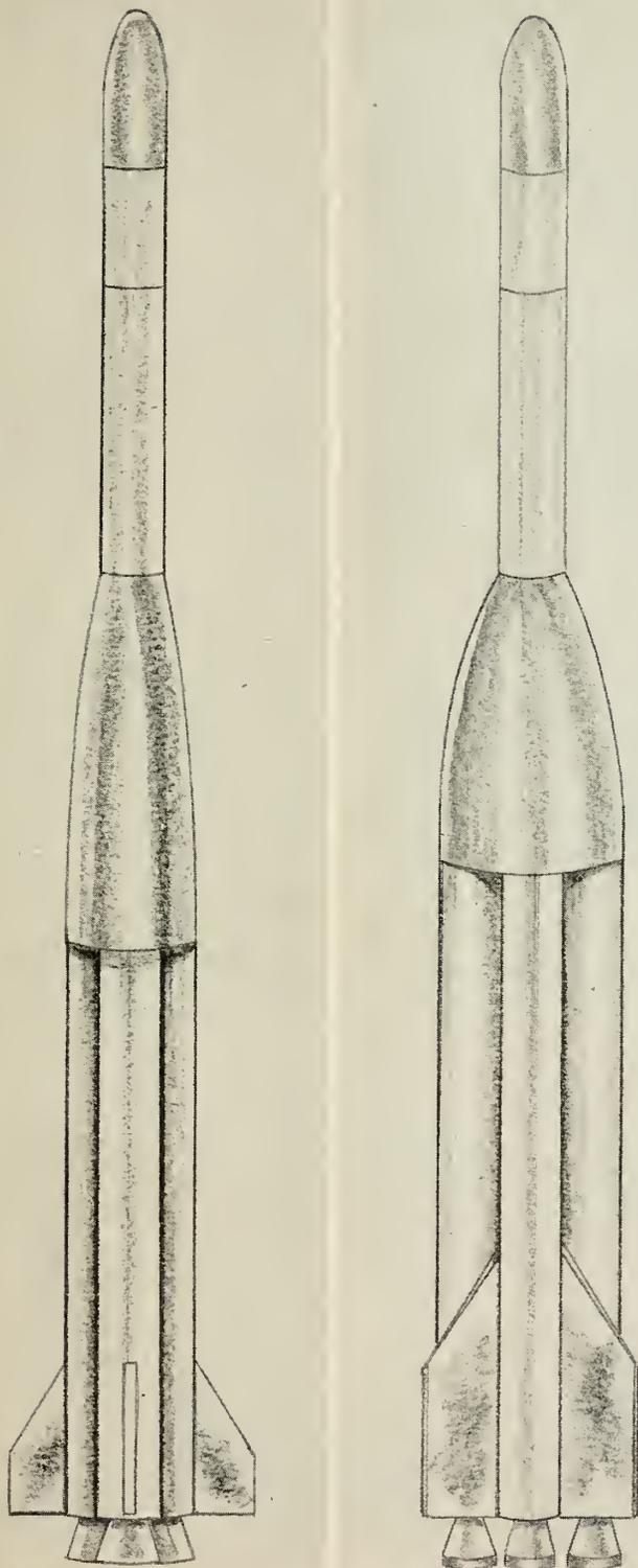
Shown in an artist's conception are possible staging arrangements for the POLARIS test vehicles. Shown are an 800-mile test vehicle (left) and a 1500-mile version (right).
