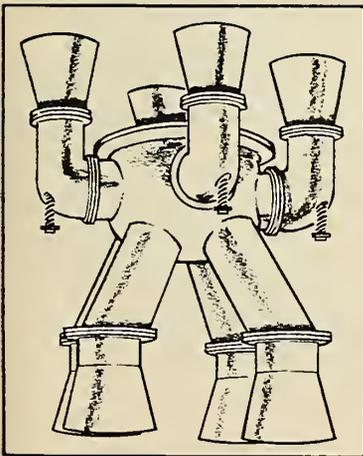
This plenum chamber with eight nozzles shows how some of the solid-propellant thinking is going at Thiokol Chemical Co. Four reversing nozzles could be used for either pitch and yaw control, clean separation or both.
