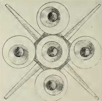
Aft view of the booster section of a possible arrangement for a 1500-mile POLARIS test missile. Center rocket could either be second stage of three-stage configuration or fifth booster rocket of possible two-stage model.
