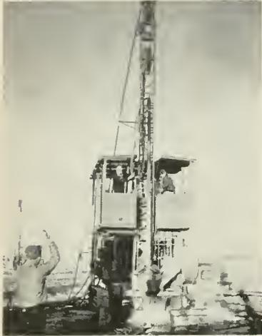
The Jet-Piercing rig is fed 10,000 cu. ft. of oxygen and 40 gal. of fuel oil per hour. Oxygen is supplied from a trailer holding enough for eight to ten hours operation.
