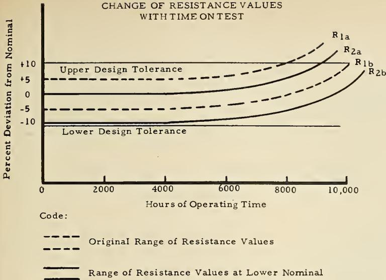
Figure 4. Change of resistance values with time on test.
