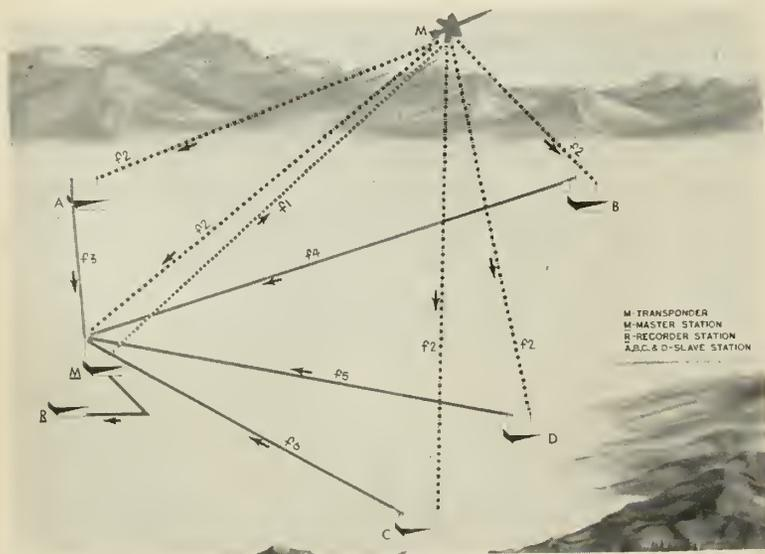
Radar triangulation pulse time system. Pulse-modulated carrier is frequency shifted in missile. This signal is again shifted by slave stations and sent to master station.
