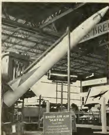
SS 10 (above left) and SS 11 (left) are surface-to-surface antitank, antiplacement missiles powered by a solid rocket motor. Missiles are controlled by transmitting signals through two wires which unwind from a drum. The MATRA 510 (above) is an air-to-air missile powered by a two-stage solid rocket motor. Missile carrier is the TRIDENT.
