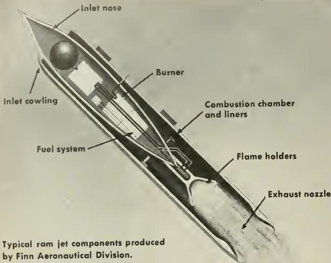
Typical ram jet components produced by Finn Aeronautical Division.
