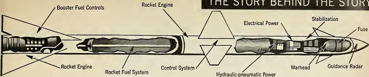
**THOUSANDS OF "FAULTS"** can develop in a guided missile, each capable of causing it to misfire or swerve off-course. Pre-launching
