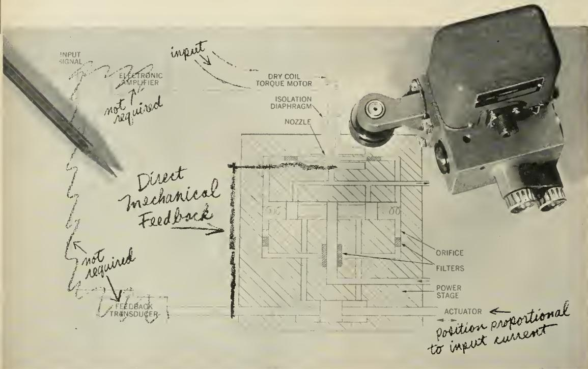
Hydraulic Research's new integrated electro-hydraulic servo valve - actuator combination eliminates amplifier and electrical feedback by the addition of a mechanical feedback spring and increased servo valve gains.
