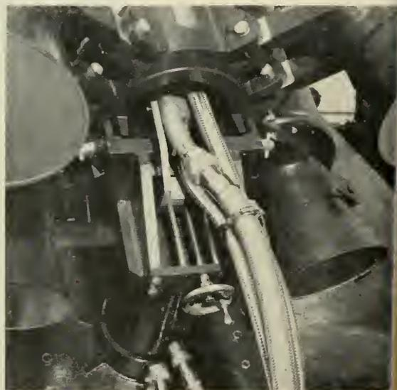
This aft view of BLOODHOUND shows hinged assembly ring of wrap-around boosters as well as hydraulic and pneumatic fittings.
