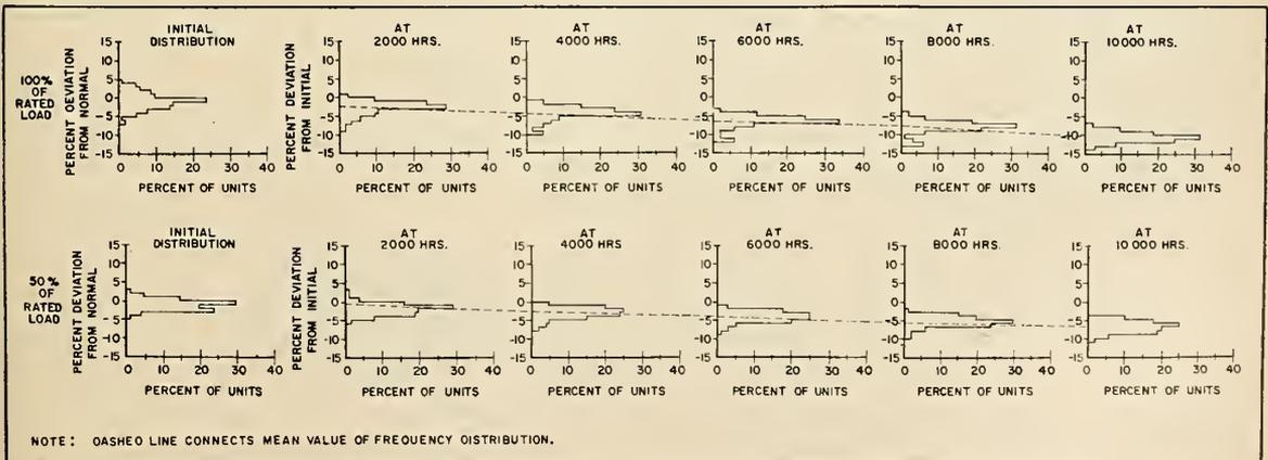
Figure 5. Per cent deviation in component characteristic for operation at 100 per cent and 50 per cent of rated load.
