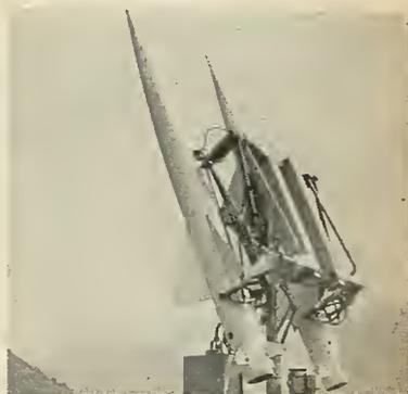
*Oerlikon's type 54 SAM, over 19 feet long, is regarded as one of the world's best antiaircraft missiles. The type 54 is a beam-rider and utilizes a liquid propellant engine burning white fuming nitric acid and kerosene. The beam-transmitter of the type 54 system is shown on the cover of missile electronics (following page 156) and has both coarse-beam and fine-beam guidance.*
