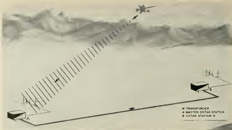
Interferometer system similar to MINITRACK, using two stations to measure phase difference at multiple antennas. Two-station system gives position, velocity, acceleration.
