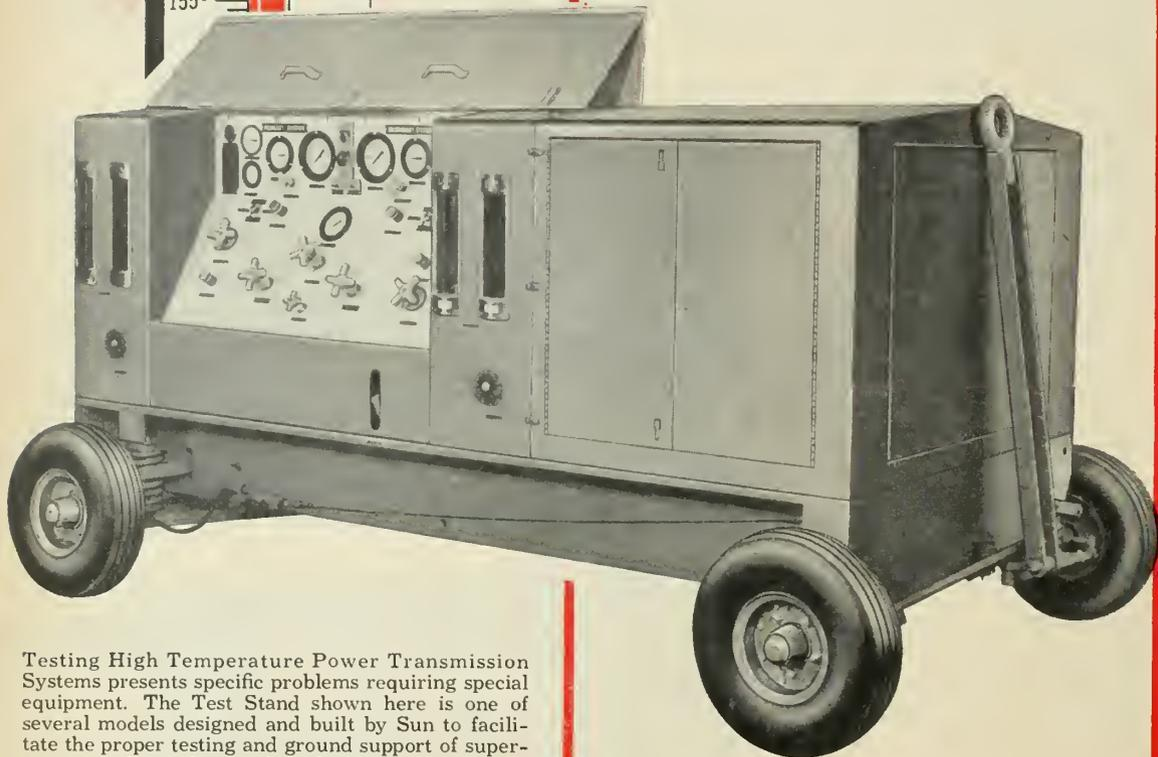
Testing High Temperature Power Transmission Systems presents specific problems requiring special equipment. The Test Stand shown here is one of several models designed and built by Sun to facilitate the proper testing and ground support of supersonic missiles and aircraft hydraulic systems.
