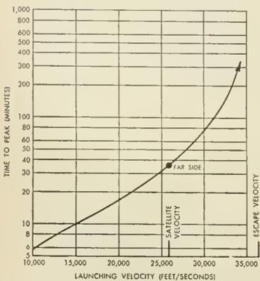
Figure 1. Parameters of FAR SIDE concept.
