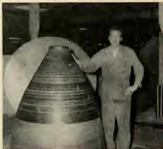
Right, cone of  $\frac{5}{8}$ " magnesium, hot spun in two parts on LEICO Model Plb 1200. Previous to new method, welded heavy or thick-walled parts caused warpage which in turn required an inside and out operation. The machines are now being used in many parts of U.S.A.
