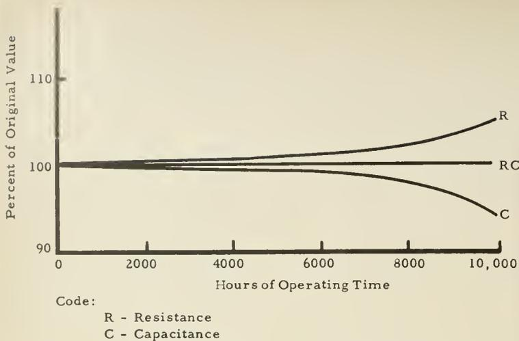
Figure 6. Drift trade-off in R-C circuit.
