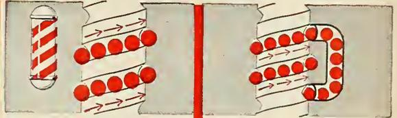
Nut glides on steel balls. Like stripes on a barber pole, the balls travel toward end of nut through spiral "tunnel" formed by concave threads in both screw and mating nut.
