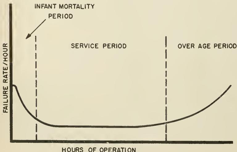
Figure 1. Component failure rate vs. operating time.
