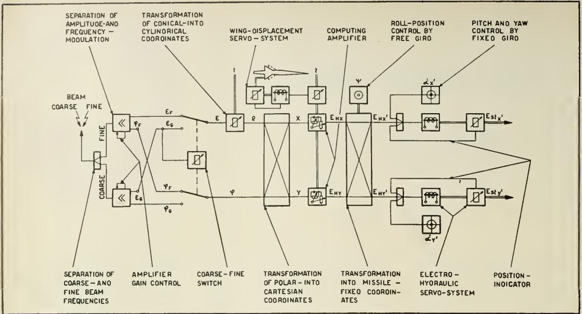
Above is a schematic diagram of the Oerlikon rocket control system showing the main components and their relationship to one another.
