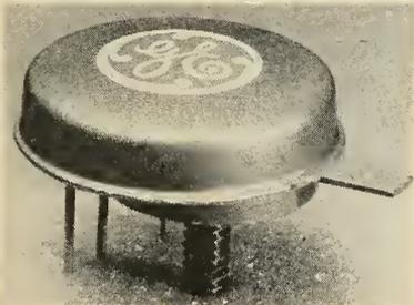
temperature transistor in the industry. The device will dissipate 85-watts at 25°C mounting base temperature and has a nominal collector saturation resistance of 2 ohms.
