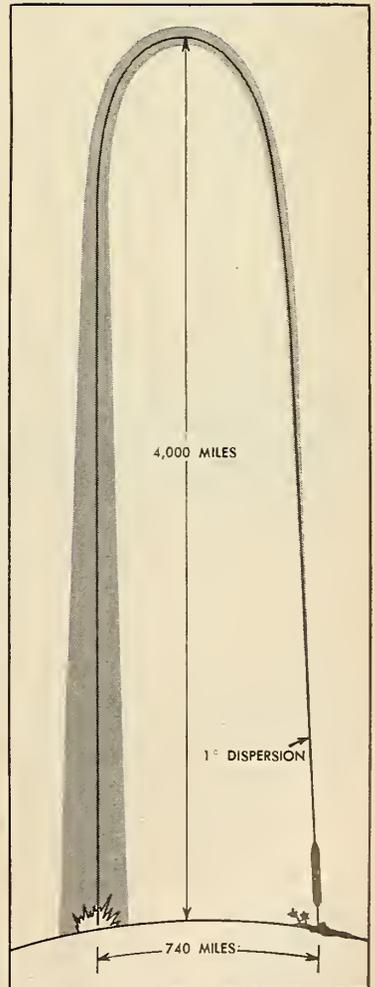
Figure 3. Trajectory of 4000-mile FAR SIDE rocket.
