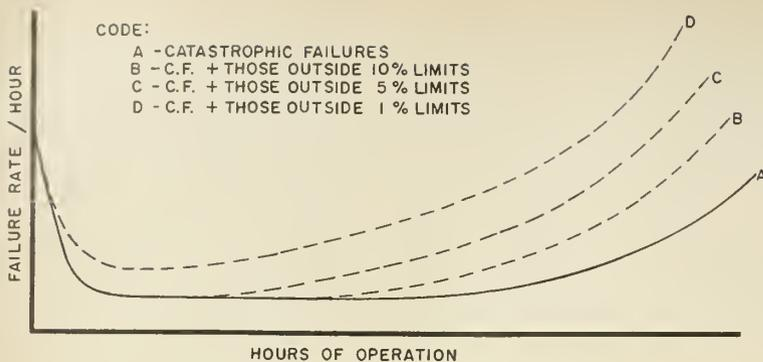
Figure 2. Component failure rate per hour.
