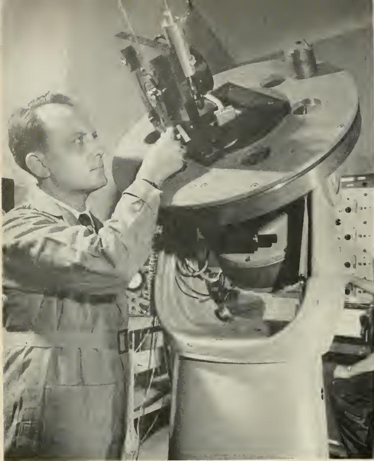
Engineer installs an air-bearing gyro on sensitive equatorial test stand in FICO test lab.
