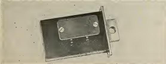
Zone box adapter (part no. 91-102-0) permits easy, precise adjustment of thermocouple reference to point desired. Adapter suitable for operation into low- or high-impedance instrumentation. Both adapter and zone box are manufactured by Magnetic Research Corporation to ABMA specifications.
