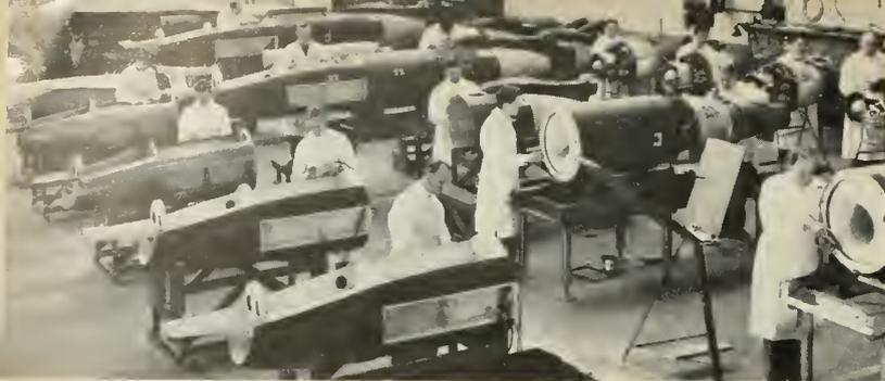
The French Air Force CT 20 in the assembly area of the SNCA du Nord manufacturing plant. The CT 20 is one of the most advanced target missiles now in production in France.
