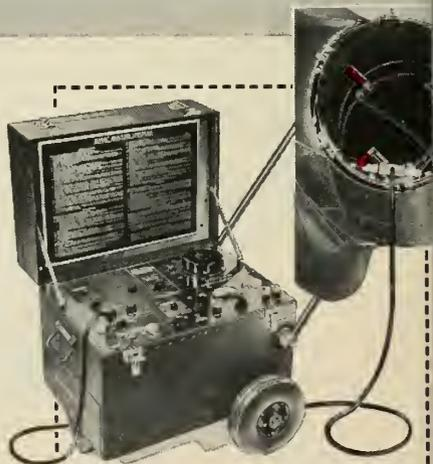
**Tests EGT System Accuracy to  $\pm 4^{\circ}\text{C}$  at Test Temperature**
