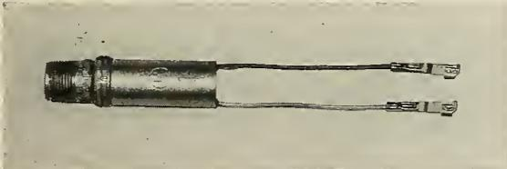
Compact, inexpensive "zone box" (part no. 91-101-0) does away with icebaths and ovens by simulating exact reference temperatures electrically. Box mounts near thermocouple, thus eliminating long leads. It withstands extreme environments without losing accuracy. Since each thermocouple feeds into its own zone box, referencing is decentralized, system reliability and flexibility are further increased.
