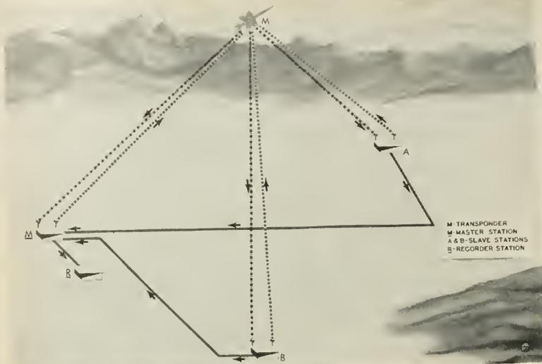
Phase measuring system. Stations send and receive a signal in sequence. Phase shift is proportional to change in path length. Station gets independent readings.
