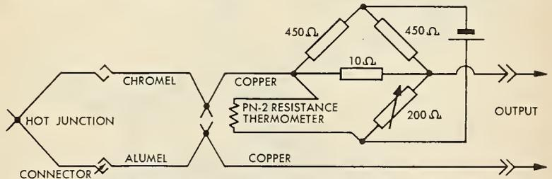
Fig. 1—Circuit diagram of first reference junction system for the REDSTONE missile. The ambient-temperature-sensing thermometer dictates proper correction into the system.
