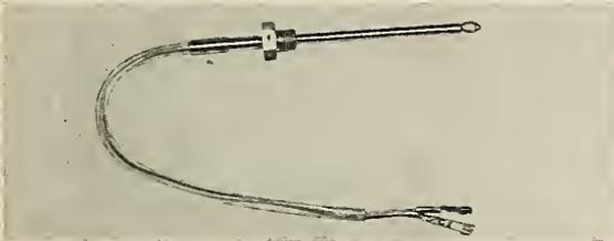
Use of thermocouples as sensing elements boosts measurement level from 900°C to a new maximum of 2000°C. Characteristic ruggedness of thermocouples also increases system reliability. Thermistors or resistance thermometers may also be used as system requires.
