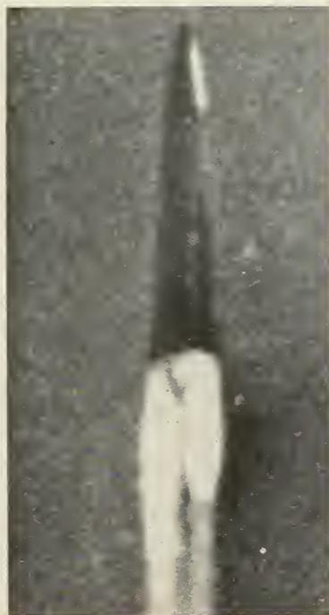
Bad news for the ICBM program—Air Force ATLAS rises above pad at Cape Canaveral in second unsuccessful attempt. The two booster engines thrust the ATLAS skyward (left). At 5000 ft. it makes tilt to east, flame increases, and seconds later it explodes.
