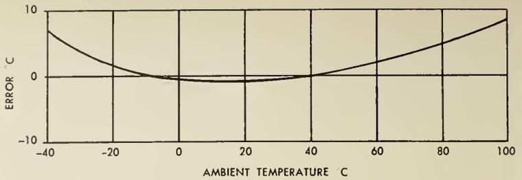
Fig. 3—Circuit diagram of "zone box" and graph illustrating the error of improper tracking of the reference thermocouple output.
