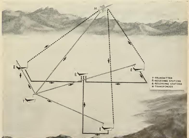
Electronic trajectory measuring system using Doppler effect. In missile, signal is doubled in frequency and sent to receiving stations for analysis at different positions.
