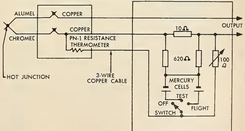
Fig. 2—Circuit diagram of an improved reference junction system for the REDSTONE. Dependability of the system is largely a function of the stability of the mercury cell.
