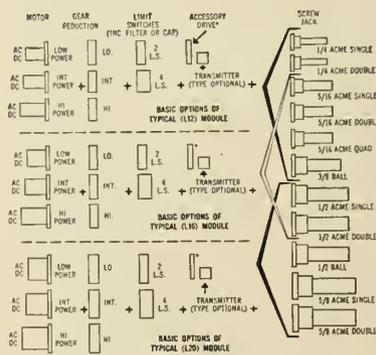
Above, the complete line of Airborne modular actuator components.
