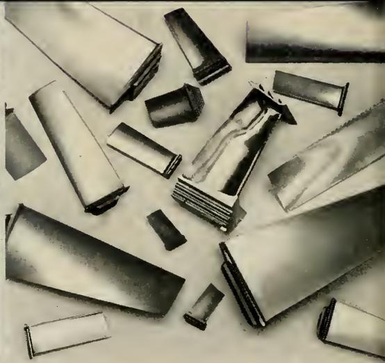
Our experience includes the precision-forging of thousands of jet engine components, with tolerances as close as  $\pm 0.003''$ .
