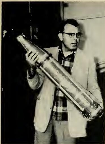
Sealed in polyethylene to protect it from the elements, EXPLORER I is carried from instrumentality checkout trailer to gantry for mounting on fourth stage of the rocket configuration. Total electronic payload weight was approximately 11 pounds, total payload 17 pounds.
