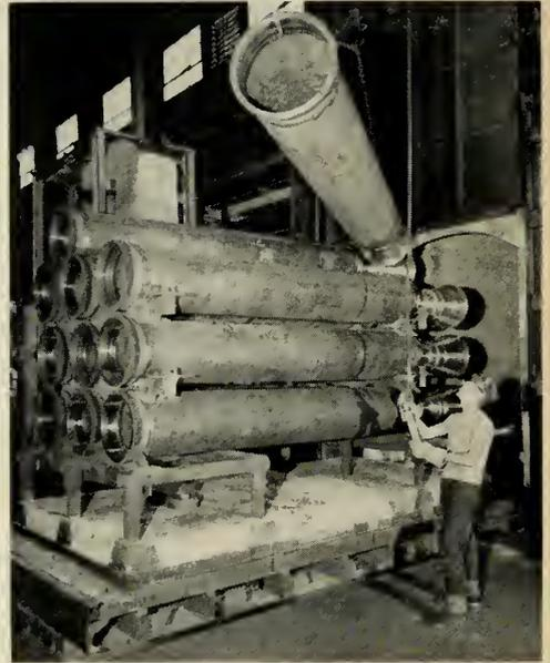
Stresses produced by the welding operations are then relieved in a furnace (Above right). To correct any misalignment which may have been caused by welding or heat-treating steps, rockets are given final thrust alignment cuts on a tracer lathe (Right) plus final alignment for fin attachment rings. Rocket motors which have been through operation show bright rings around nozzle (Below).
