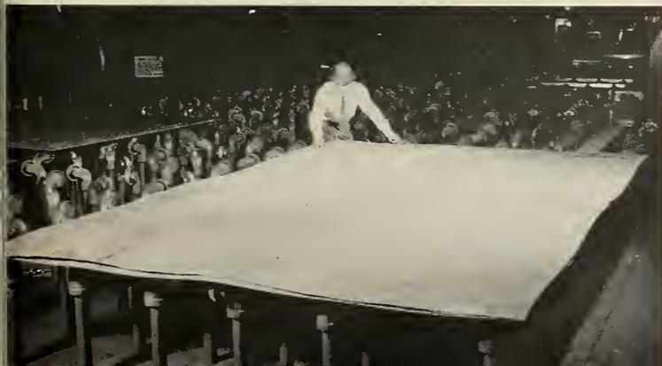
Above—Workman at Homestead Works coating stainless-steel plate with a special separating compound during the assembly of carbon-steel and stainless-steel "sandwich." Use of this compound prevents fusing of the metal plates during the hot-rolling process. After rolling, ends and sides of the carbon plates are sheared away; the resulting stainless plates are the widest ever produced on existing mill equipment. Left—Inspector examines finished stainless sheets after rolling.
