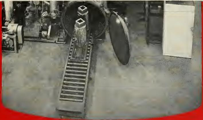
● Maximum strength can be provided in vacuum-melted, vacuum-cast super-alloy investment castings produced by Kolcast from ingot to finished part. Unique Kolcast equipment and exclusive methods keep super-alloy melts and castings free of oxygen and other strength-sapping gases.
