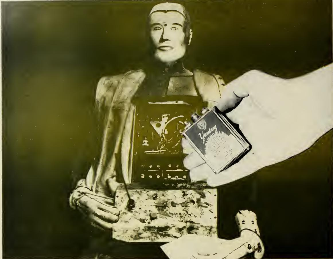
To perfect supersonic escape techniques, the Coleman Engineering Company has created Hurricane Sam, an amazingly real 6-ft., 180-lb. "man". Internally, a YARDNEY SILVERCEL® Battery—a power pack smaller than a human heart—runs strain gauges, accelerometers and a telemetering transmitter, that measure
