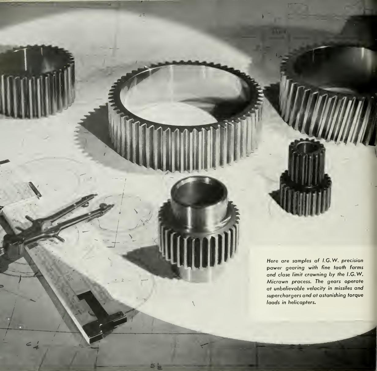
*Here are samples of I.G.W. precision power gearing with fine tooth forms and close limit crowning by the I.G.W. Micrawn process. The gears operate at unbelievable velocity in missiles and superchargers and at astonishing torque loads in helicopters.*
