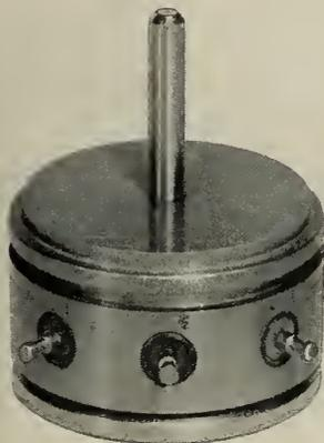
desired shape on the prepared surface of the ceramic base or "substrate." Thickness of the coatings can be controlled to produce accurately the desired electrical characteristics. The entire process can be accomplished by the use of fully automatic equipment.
