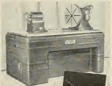
The heavy duty dividing head is built to handle work with a swing up to  $24\frac{1}{16}"$  dia. Surface plate is  $36" \times 72"$ . This model has the same accuracy as the standard model.
