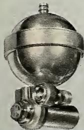
Gas generator pressurizes hydraulic accumulator — can also drive turbines, operate pneumatic servos, provide jet thrust, give instant power for any requirement.
