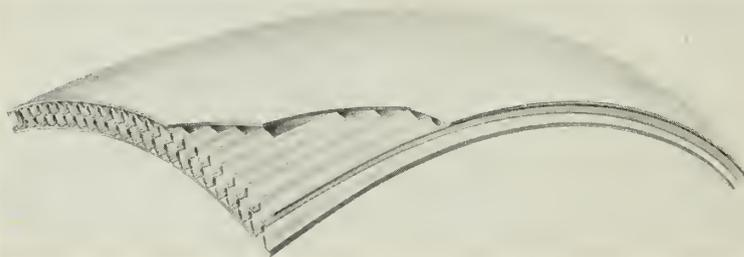
Welded stainless steel—double "vee" corrugation.
