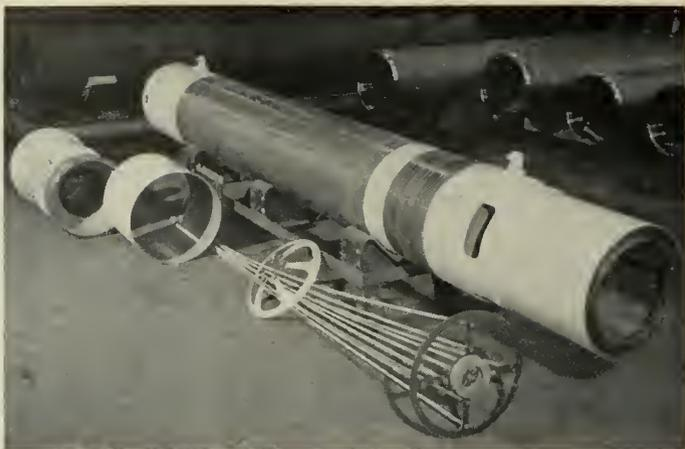
A plastic-impregnated, fiberglass NIKE rocket, manufactured by Goodyear while investigating better ways to make the boosters.
