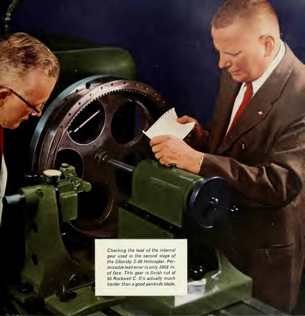
*Checking the lead of the internal gear used in the second stage of the Sikorsky S-58 Helicopter. Permissible lead error is only .0003 in. of face. This gear is finish cut at 50 Rockwell C. It's actually much harder than a good penknife blade.*
