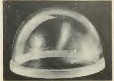
considerably more than a hemisphere, and in aspheric shapes. Physical dimensions are controlled during manufacture to achieve extremely close tolerances. After final grinding and polishing, spherical tolerances are held to millionths of an inch, diameters to ten thousandths, and concentricity between inner and outer surfaces within ten thousandths.
