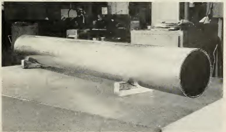
Single "vee" resistance-welded stainless-steel hollow-core tube may have rocket uses.
