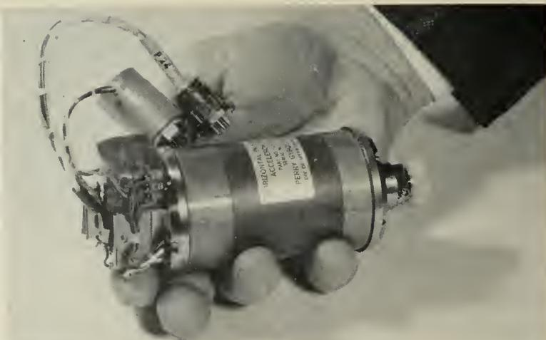
nent of acceleration along its longitudinal axis moves the sensor along this axis for precise electronic measurement.
