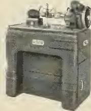
Model 55—38 is available either with a  $20" \times 40"$  surface plate; capacity between work centers 22", or a  $20" \times 72"$  surface plate; capacity between work centers 54". Both have a work swing of  $12\frac{1}{2}^{\circ}$  dia.
