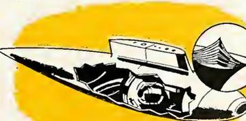
SOLAR AIRCRAFT COMPANY'S gas turbine A.P.U. pod had to take oven-hot temperatures up to 400 F... contact with oil and gas fumes... rough ground abuse... aerodynamic loads... severe runway abrasion from its underslung position. So Solar engineers designed a laminated pod of tough, lightweight Conolon® 506. The extra-tough pods, assembled on inexpensive molds, have demonstrated their ability to "take it" after hundreds of hours of flying time.
