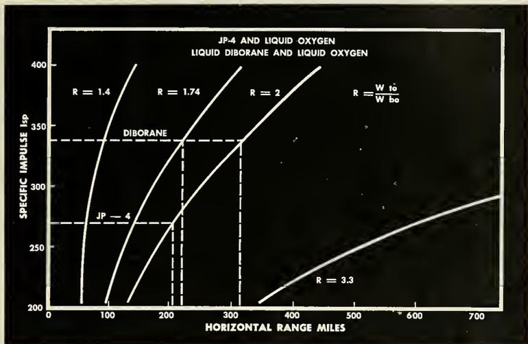
RANGE PERFORMANCE of a hypothetical rocket vehicle with JP-4 and liquid diborane compared. Diborane would require larger tank.
