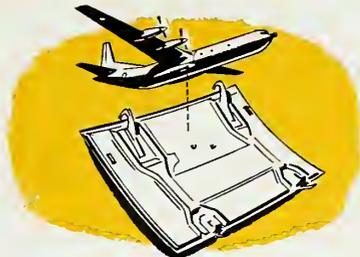
WHEN DOUGLAS AIRCRAFT CO. engineers faced the problem of attaching hardware to sandwich access doors of the C-133A transport, they solved it by using Narmco Formula 3119 Putty plugs. This easy-to-use, room-temperature-setting putty was cast in place and drilled for bolts and blind fasteners. In shear tests, both skins and core failed before the putty-supported attachments.
