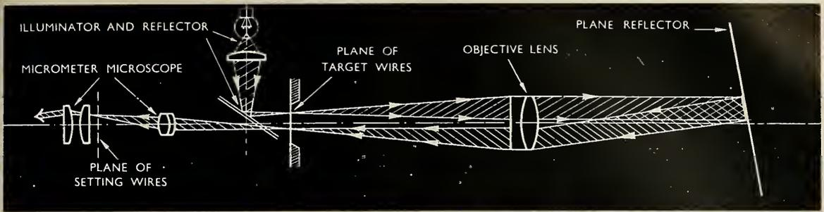
A MICROOPTIC AUTO-COLLIMATOR consists of a telescope with a pair of cross-wires set in the focal plane of the objective lens and illuminated. Light emerges from the lens as a parallel beam, and projects onto a plane reflecting surface. The reflected beam is received back into the optical system, forming an image of the cross-wires in the same plane as the cross-wires. Displacement of the image is measured to an angle of tilt of the reflecting surface, as little as 1/10 second of arc.
