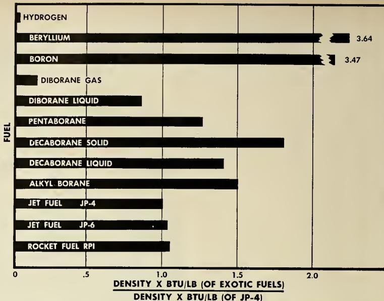
**CHARACTERISTICS** of the borane fuels show that low density of diborane adversely affects its mass ratio and offsets the theoretical increase in  $I_{sp}$ .
