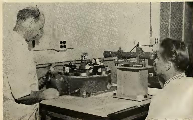
**TECHNICIANS** from Northrop Aircraft check high-precision missile gear with Watts Microptic Rotary Table and Watts Microptic Auto-Collimator. The Auto-Collimator is sighted into surface mirror, attached to the spindle of the table at the fulcrum point of a master work gear. Variance is held within close tolerance. Tolerance buildup in conventional gears causes serious problems in missiles.
