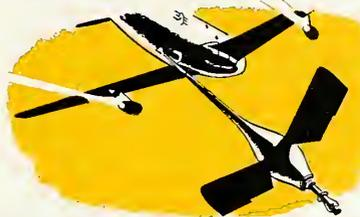
THIS "RUDDEVATOR"—a bonded sandwich structure—for the Boeing KC-135 jet tanker's flying boom required a structural adhesive capable of withstanding severe loads as well as enormous operational punishment. The solution: Narmtape® 102 system, a supported adhesive formulated with non-brittle constituents to provide unmatched fatigue resistance under highest stress and vibration.
