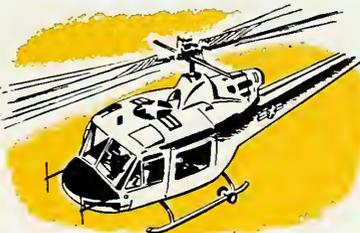
BELL HELICOPTER engineers achieved weight savings... fabrication economy... and longer fatigue life when they selected a laminated metal design for the XH-40 rotor blade, which is bonded with Narmco's Metlbond® 4021 system... distinguished for its high peel strength and outstanding resistance to fatigue. Exhaustive tests have shown that bonded rotor blades are able to meet demanding performance requirements under repeated flexural loads.
