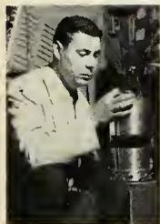
Many of the components that got their first ride on this tape-driven shaker are now circling the sky in Explorer I, our first successful earth satellite. It is highly significant that the California Institute of Technology Jet Propulsion Laboratory which led the development work on this satellite also pioneered complex-wave vibration testing. In this technique, magnetic recording plays many vital roles.
