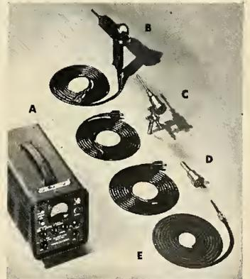
(A) Standard control unit is used with any one of the following detectors: (B) gun detector, (C) stationary detector, (D) vacuum detector, (E) pencil-probe detector.
