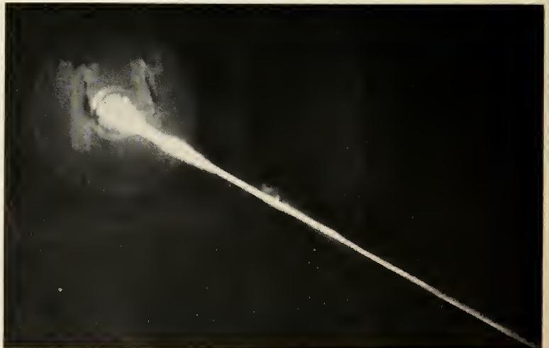
**THE EFFECT OF A METEORITE PUNCTURE** of a neon-gas-filled satellite would be similar to that shown in this NACA photo. The radiation belt surrounding the earth would act on the neon and make it glow as it rushed from the satellite. Deliberately releasing large quantities of neon in this belt would cause a large glowing area in the sky and permit observation and measurement of the area.
