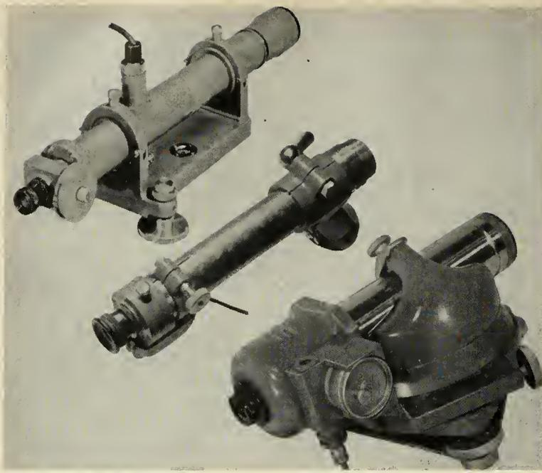
FROM TOP LEFT: Watts Microptic Auto-Collimator, Hilger and Watts angle Dekkor, and Taylor-Hobson Auto-Collimator. Eyepieces and micrometers are sealed to read the angle of file on the reflector directly.
