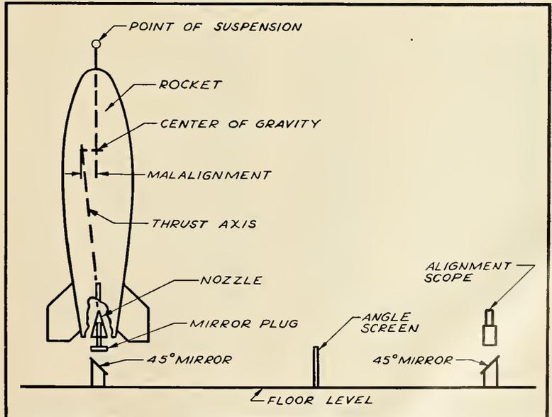
ALIGNMENT TELESCOPE measures thrust-to-rocket-axis by means of angle screen and mirror plug. Accuracy is on the order of an angle of 1 minute, 15 seconds.
