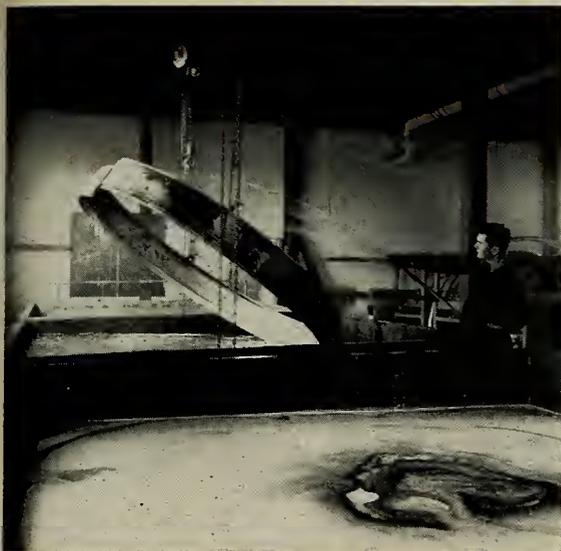
**CLEANLINESS** is an absolute necessity, not only to assure structural integrity, but to preclude any contamination of the liquid oxygen. Here oxides are removed prior to welding.
