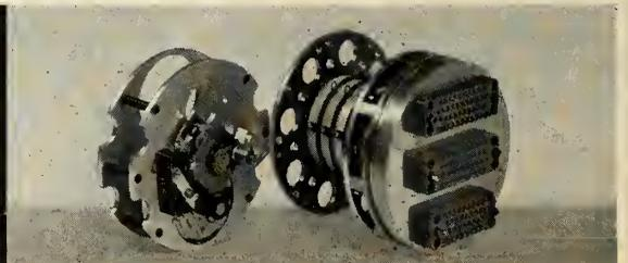
**Ground Power Changeover Control**—This assembly (airborne) provides remote control of the transfer from external to internal bird power. Of compact and efficient design, its multiple-contact circuit breaking design allows more than 2 amp and 500 VDC capacity with ample margin. Partial assembly only, shown.
