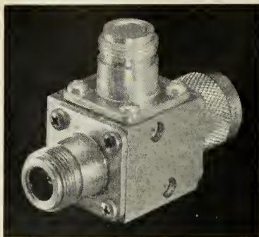
A diplexer designed to isolate the S-band from the X-band has been introduced by Microphase Corp. In the S-band, the insertion loss is less than 1.0 db, while in the X-band it is under 1.5 db. The isolation is a minimum of 30 db.
