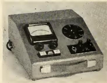
closing and opening times of relays, circuit breakers and snap switches.
