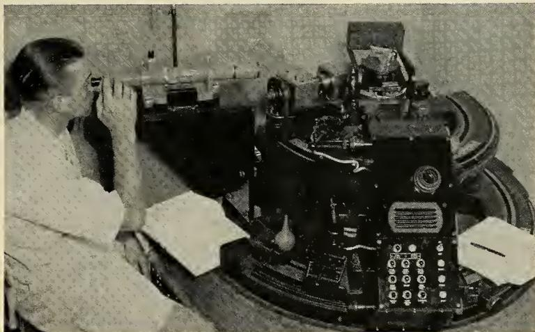
**INSPECTION OF PRECISION MISSILE GEARS** at Northrop Aircraft comprises a primary and secondary optical system. This allows a two-way check of the indexing system, and holds it to a tolerance of 1/10 second of arc (half a millionth of an inch per inch). The operator is shown using an auto-collimator to readjust the machine's calibration every 7½ degrees of carriage travel to correct any accumulative error. This installation is perhaps the most accurate indexing system in use in the U.S.
