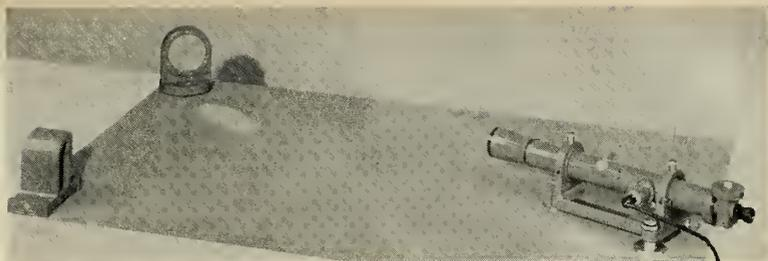
**CHECKING SURFACE PLATES** for flatness. Here is a typical arrangement. A Watts Microptic Auto-Collimator, corner mirror, and mirror carriage is moved along the line being read for flatness. Demand for more and more precision in missile engineering today makes laboratory equipment, such as surface plates, a critical item in measurement and check-out of precision components.
