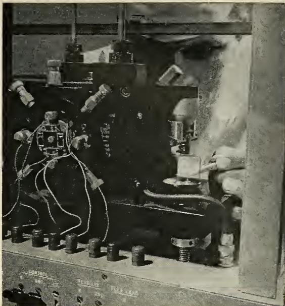
**M-H TORQUE BALANCE DEVICE** used to calibrate micro-syns. It measures torques as low as one eight-billionth of a lb.
