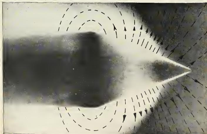
**WITH MAGNETIC FIELD.** Here is shown the magnetohydrodynamic displacement of the shock wave. The magnetic field is caused by electric current flowing through a coil of wire within the cone. This experiment qualitatively demonstrates the interaction of a high-temperature gas with a magnetic field. This effect would be expected to produce drag and reduce heat transfer to the body.
