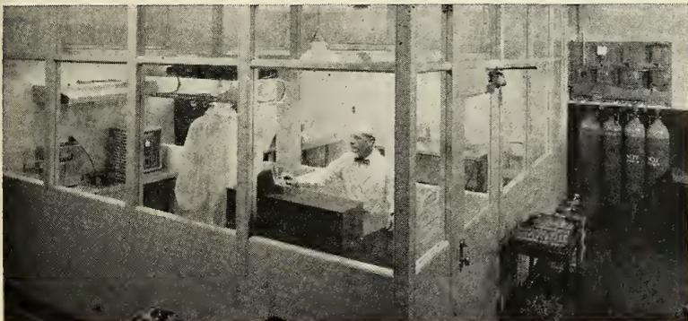
"Clean room"—working areas with controlled, dust-free atmospheres—aren't limited to the guidance manufacturers. The Superior Valve and Fittings Co. of Pittsburgh recently placed in operation a 16 x 16 ft. room for processing precision valves and parts for missiles.
