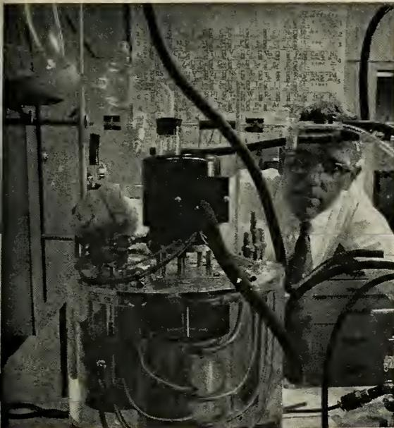
**MATERIAL LABORATORY** is scene for testing gas solubility of flotation fluid for new type liquid-floated gyroscope.
