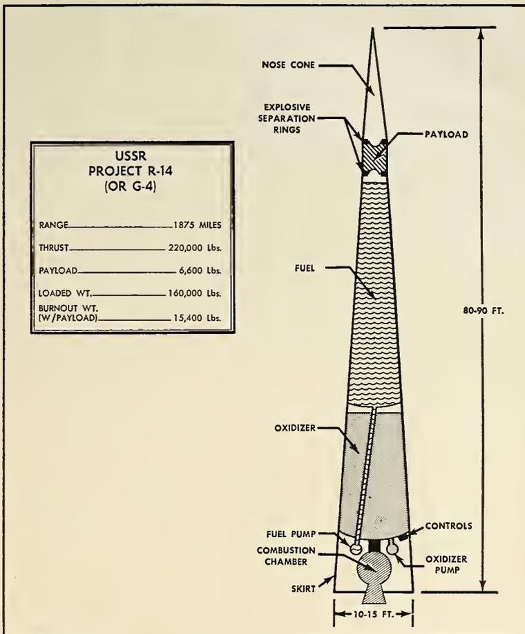
and short burning time. Accuracy of placing the 6,600 lb. warhead on target was to be 1% of the range and azimuth.
