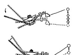
CLASSICAL IMC ENTIRE SPACECRAFT TURNS TO TRACK TARGET - BREAKS COMMUNICATIONS LINK WITH EARTH
