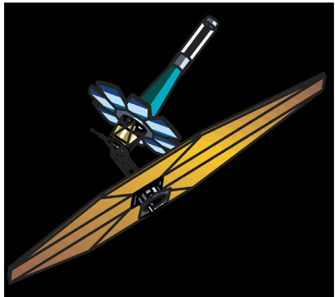
An early concept for the James Webb Space Telescope – known at the time as the Next Generation Space Telescope – was designed by a Goddard Space Flight Center-led team. It already incorporated a segmented mirror, an “open” design, and a large deployable sunshield.
