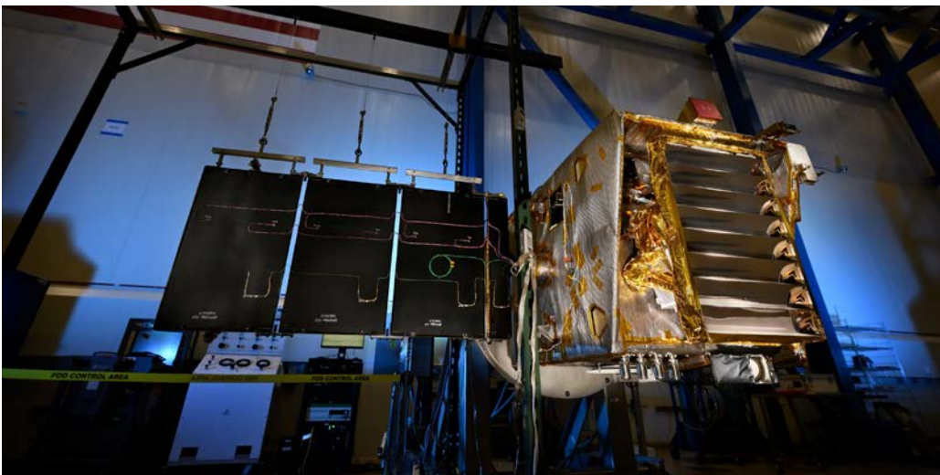
Lunar Trailblazer in a clean room after undergoing environmental testing at Lockheed Martin Space. One of two solar panels deployed.
