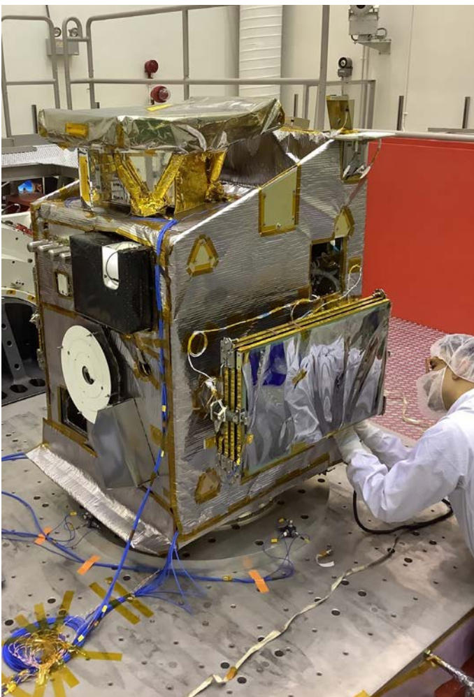
NASA's Lunar Trailblazer sits in a clean room at Lockheed Martin Space in Littleton, Colorado, as an engineer prepares the spacecraft for vibration testing.
