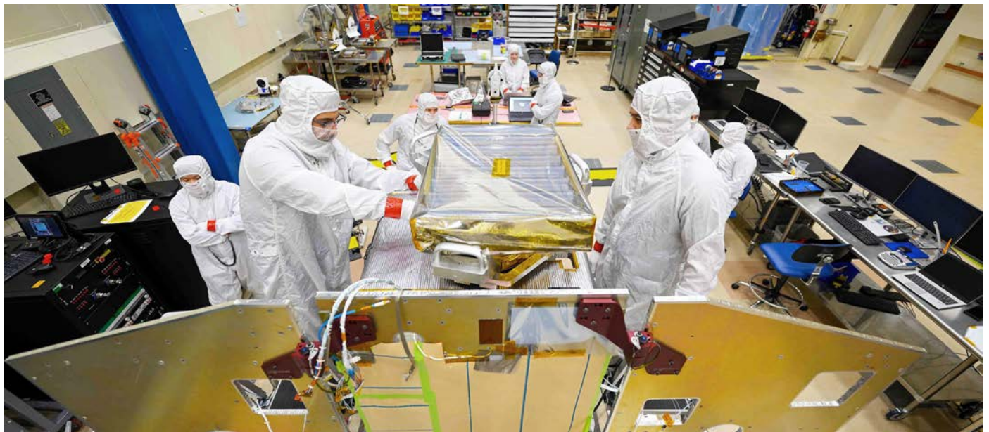
Engineers install the JPL-developed High-resolution Volatiles and Minerals Moon Mapper (HVM 3 ) for NASA's Lunar Trailblazer spacecraft in a clean room at Lockheed Martin Space in Littleton, Colorado, in December 2022.
